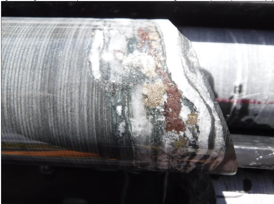
Figure 4 - ONGDD_004 Diamond Core at 574.5m with Chalcopyrite (Cu), Sphalerite (Zinc) and Pyrrhotite in Quartz Carbonate Veining
