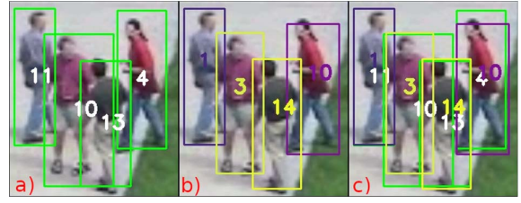
Fig 4. An illustration of the tracking exception situation i): a) YOLOv3 detections in the frame F_k (marked with light green colour); b) the bounding boxes of active trackers in the frame F_{k-1} (marked with yellow and purple colours); c) overlapping of detections in F_k with trackers in F_{k-1} .
