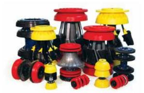
Steel-Body pigs, or Mandrel pigs, are heavy duty pigs which can be configured in a number of ways to provide maximum cleaning, sealing and sweeping power. These pigs can travel long distances and the urethane cups and discs are replaceable which makes them an economical option for many pipeline operators.
