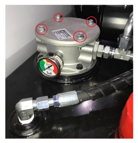
4. Remove the low pressure filter element and replace it with a K10 Filter Element (PN – HY-1300) and rebolt the filter cap to housing 5. Remove the red colored Pressure Filter holder (bottom portion) from the upper filter housing
