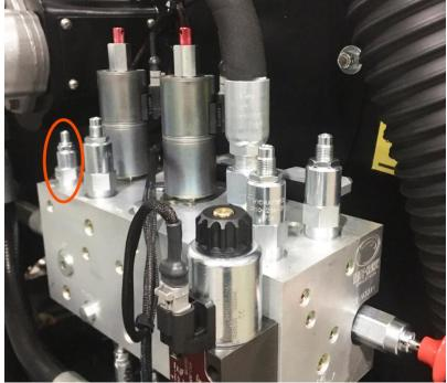
Loosen the jam nut on the relief valve and turn the screw counter-clockwise for more speed and clockwise for less. Note that this relief valve also controls the speed at which the broom extends and retracts.
