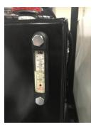
Sight Gauge (Reservoir) – if you can not see fluid in this gauge, inspect system for leaks and don't operate sweeper until fluid level is half way up the gauge. Also check fluid quality – free of contaminants
