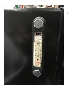
8. Refill the hydraulic reservoir to the center of the site gauge with AW 46 hydraulic fluid.
