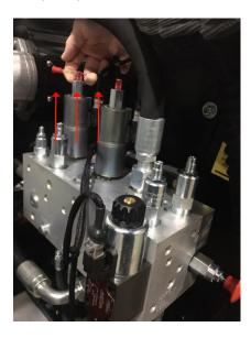
Simply push and hold down on the button to operate valve in other direction. This works for both curb broom and pickup head directional valves
