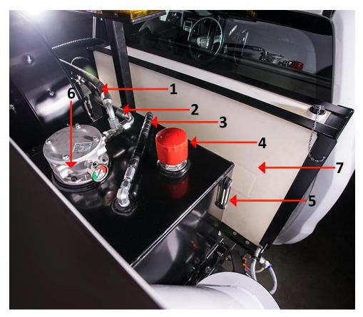
Hydraulic System Reservoir, Passenger side, Top View
