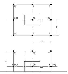
Figure 10: Prescribed Points, Medium Machine (all points of measurement shall be located on the rectilinear planes prescribed, where d is equal to 1 m or greater).
