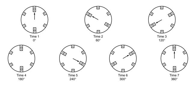
Figure 3.1.20 Magnetic Field Rotation, 3 Phase 2 Pole Motor
