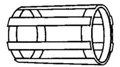
Rotor Bars and End Rings Squirrel Cage Rotor
