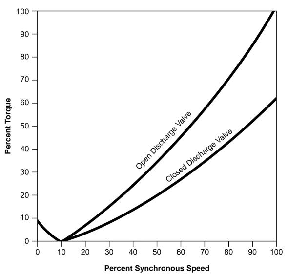
Typical Speed-Torque Curve (Centrifugal Pump)
