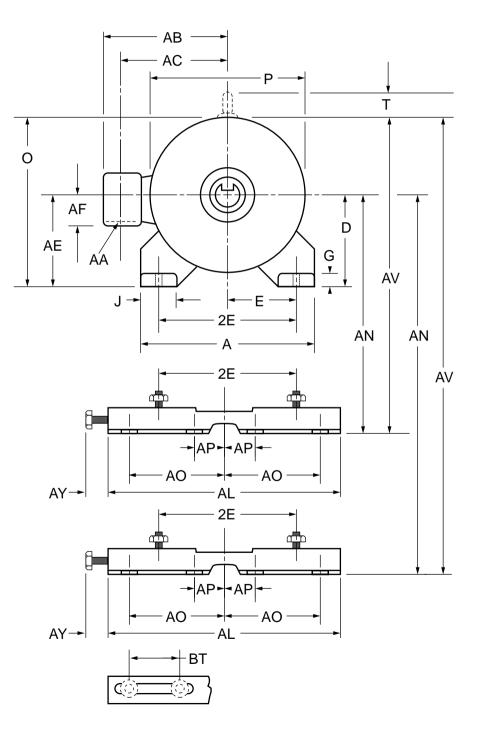
Figure 2.4.2 Lettering of Dimension Sheets for foot-mounted machines-drive end view
