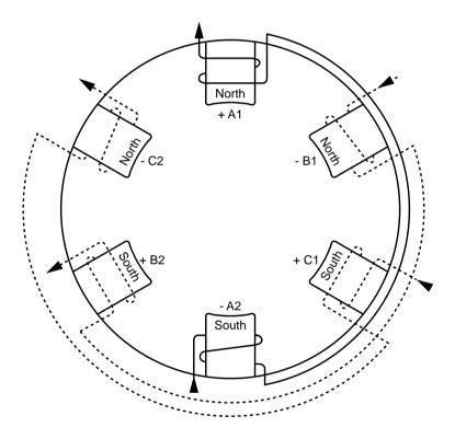
Figure 3.1.16 Coil Identification and Connection Polarity Current Flow (Direction) Shown at Time T1
