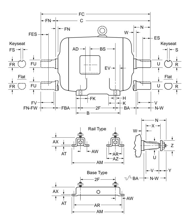
Figure 2.4.1 Lettering of Dimension Sheets for foot-mounted machines-side view
