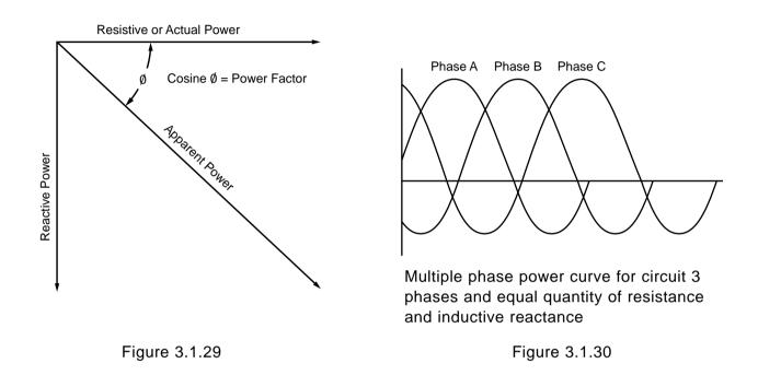
The discussion thus far concerning circuits with pure resistance or pure inductive reactance, or a combination of both has dealt with a singular source of power or single phase power. A multiple phase power supply operates in the same manner with the prime exception that the power curve tends to be smoothed out (See Figure 3.1.30).
