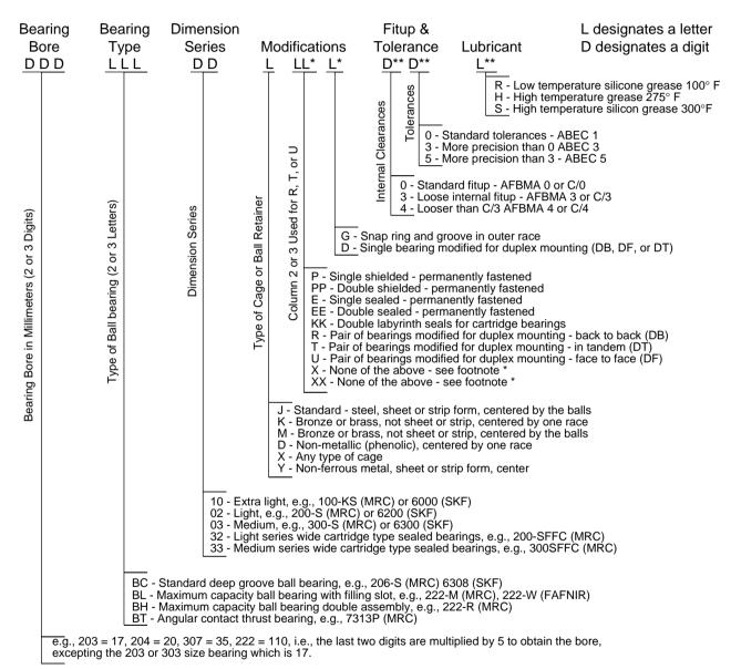
Example: 35BC02JPPO - Standard deep groove, light series, standard steel cage, double shielded, standard fitup and standard tolerances MRC 207-SFF or equivalent.
