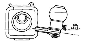
Figure 6.4.25 - Oiler and connecting pipe not level.
