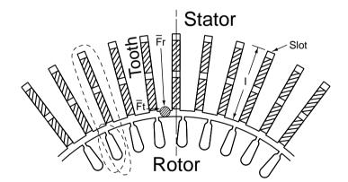
Fig. 5: Magnetic field around rotor bar and resulting forces
