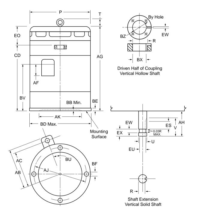
Figure 2.4.5 Lettering of Dimension Sheets for vertical machines
