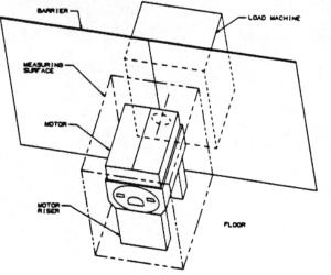
Sound intensity readings are taken at points on each of the four planes of the measuring surface.
