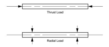
Figure 6.4.5 - Two types of loads carried on motor shafts
