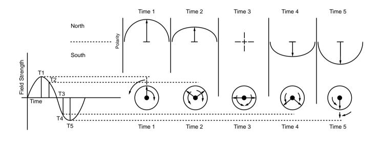
Figure 3.1.13 Field Strength with Respect to Time
