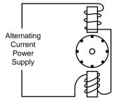
Simple Alternating Current Electric Motor
