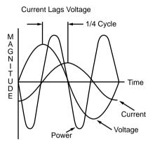
Power curve showing instantaneous valves of power for circuit having pure inductive reactance.
