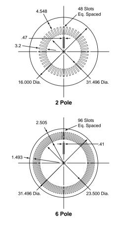
Figure 9: Comparison of two pole and six pole punching
