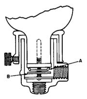
Figure 6.4.26 - Adjustment of the oil level.
