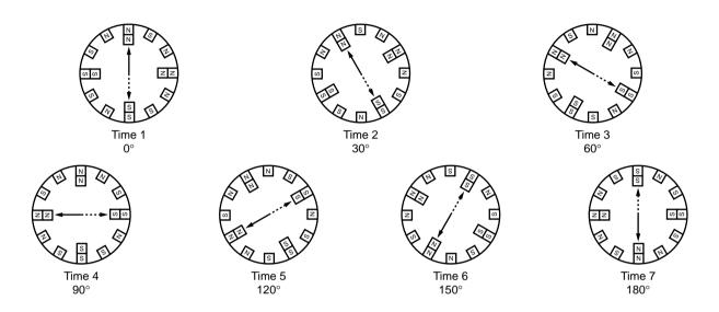
Figure 3.1.22 Magnetic Field Rotation, 3 Phase 4 Pole Motor
