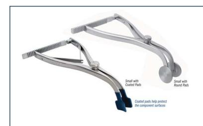
The coated spreader is designed to separate the femur and tibia when implant components are in place. This is helpful in checking the back of the knee joint for cement, etc. The pads are coated to keep from scratching component surfaces and are slightly contoured to add stability against the curved articulating surfaces.
