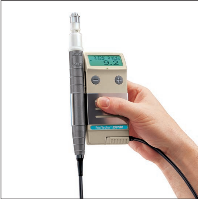
Fig. 2: A handheld digital gage for measuring air temperature, surface temperature, and relative humidity. It uses the values to calculate dew point and the difference between the dew point and the surface temperature.
