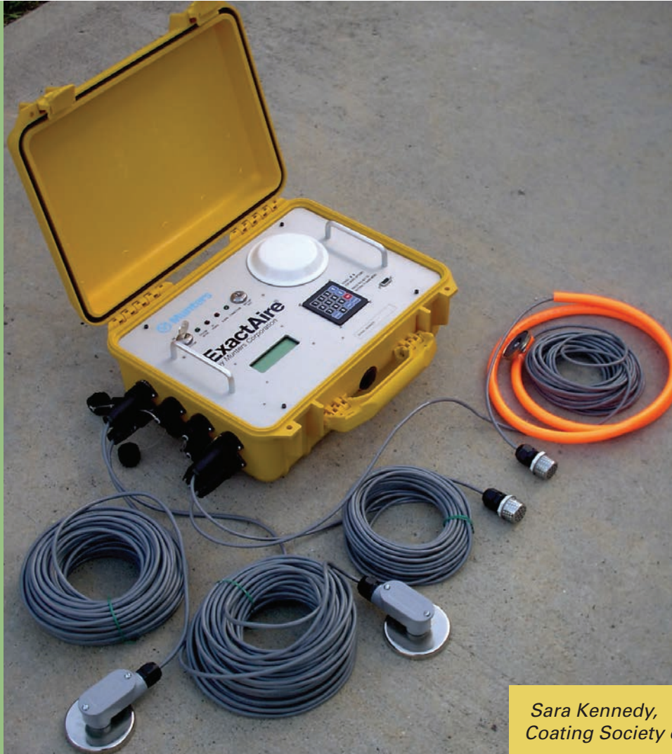
Fig. 1: Monitor with 24-hour uplink to internet with secure access allows surface temperature, ambient conditions, and dew point spreads to be checked from a remote location. Courtesy of Munters Moisture Control Services
