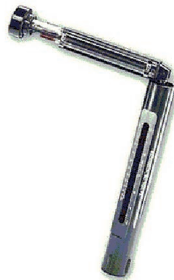
Fig. 3: A sling psychrometer (above) along with a surface temperature gage and psychrometric charts can be used to determine dew point and relative humidity. Courtesy of Bacharach
