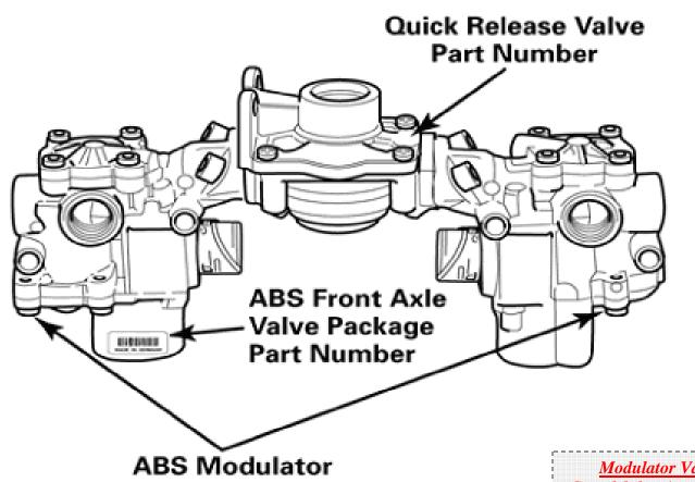
**Contains** A Quick Release Valve with Two Modulator Valves, which is mounted in the front of the vehicle near the **Brake Chambers**
