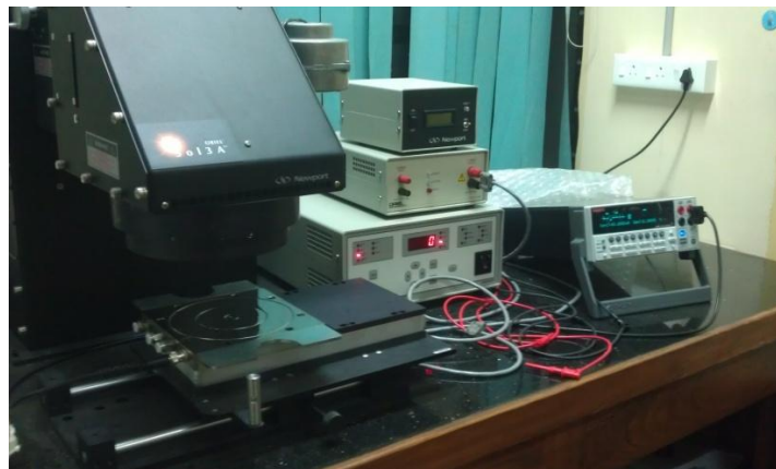
Fig. 3.30: Oriol Sol3A sun simulator used for I-V measurement
