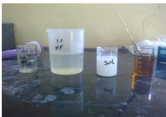
Fig. 3.6: Beakers showing the chemicals required for activation of the substrate
