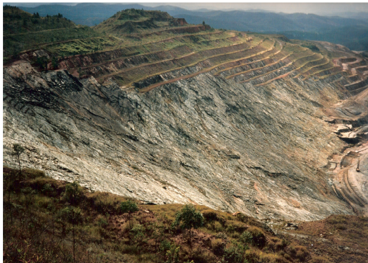
Figure 7 - Application of benches (Photo courtesy of Vale)
