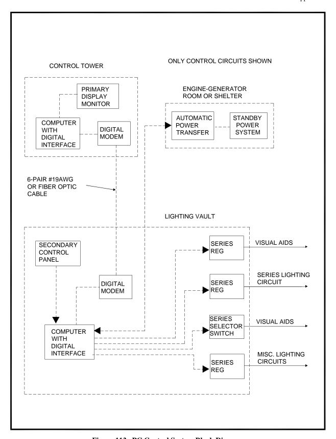
Figure 113. PC Control System Block Diagram
