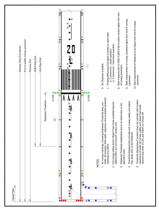
Figure 10. Lighting for Runway with Displaced Threshold not Coinciding with Opposite Runway End
