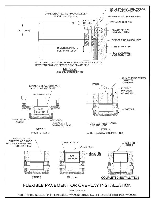
Figure 100. Flexible Pavement or Overlay Installation
