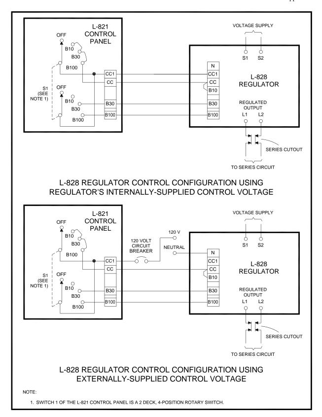
Figure 27. Alternative 120 Volt AC Remote Control System
