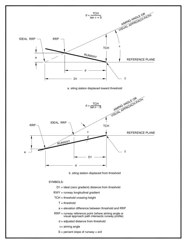
Figure 82. Correction for Runway Longitudinal Gradient
