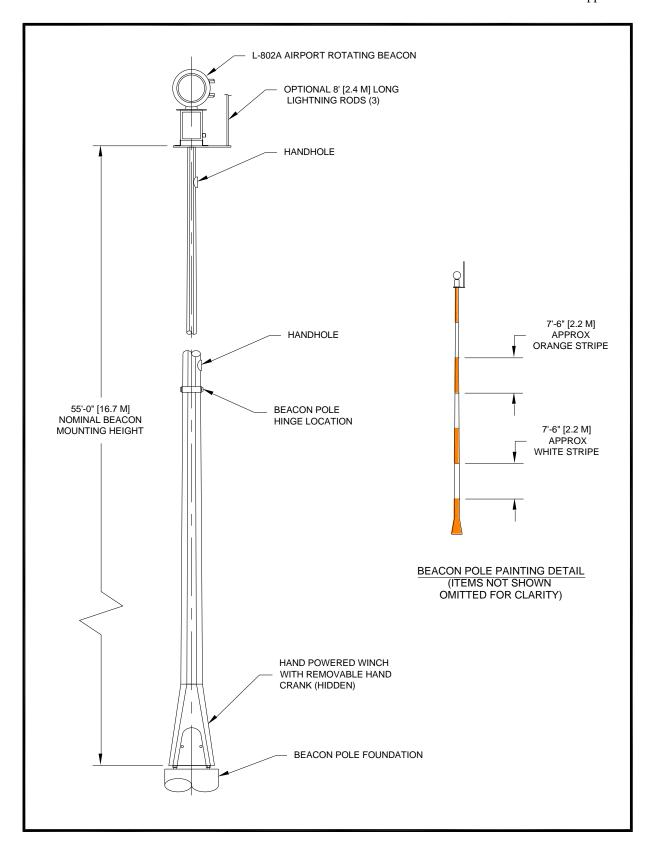
Figure 73. Typical Airport Beacon Tip-Down Pole
