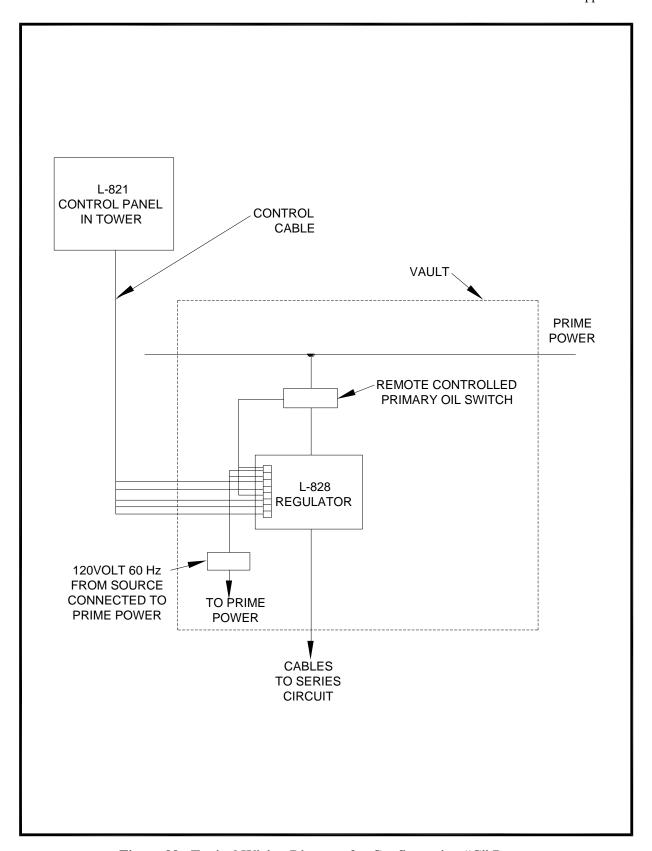
Figure 99. Typical Wiring Diagram for Configuration "C" Power
