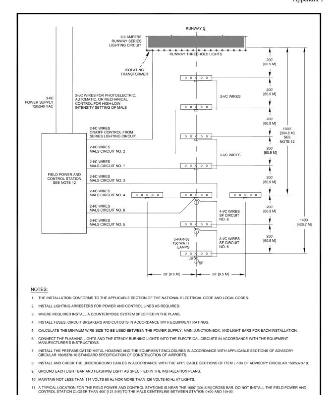
Figure 85. Typical Field Wiring Circuits for MALSF
