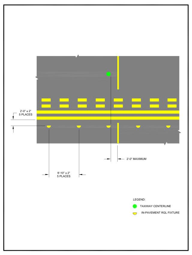
Figure 49. In-Pavement Runway Guard Light Configuration
