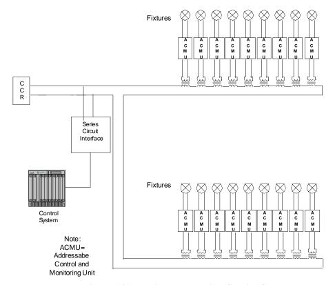
Figure 141. Typical Power Line Carrier System
