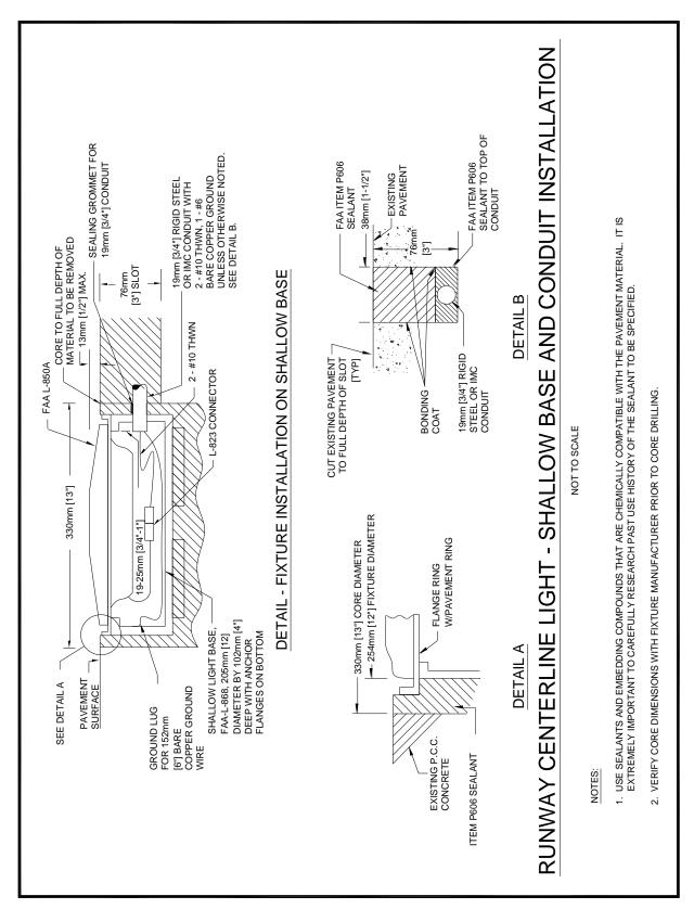
Figure 37. Runway Centerline Light - Shallow Base and Conduit Installation
