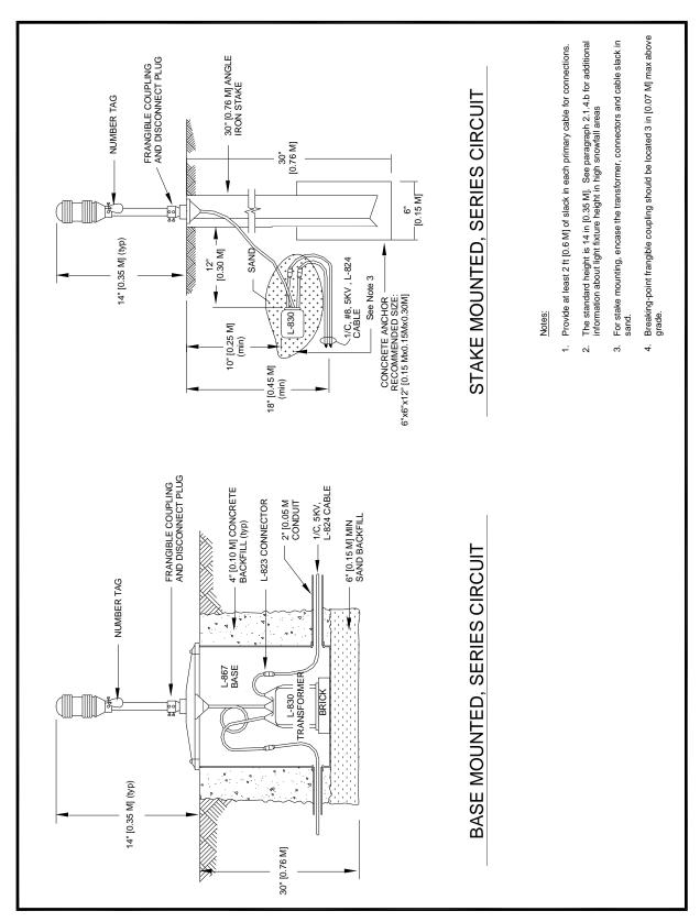
Figure 23. Light Fixture Wiring.
