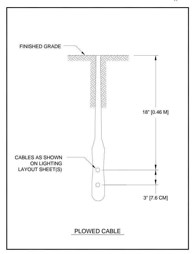
Figure 123. Standard Details for Underground Cable Installation – Plowed Cable
