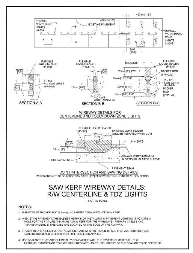
Figure 38. Saw Kerf Wireway Details
