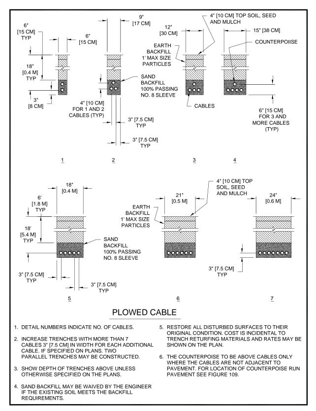
Figure 124. Standard Details for Underground Cable Installation – Plowed Cable
