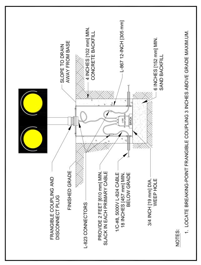
Figure 54. Typical Elevated RGL Installation Details
