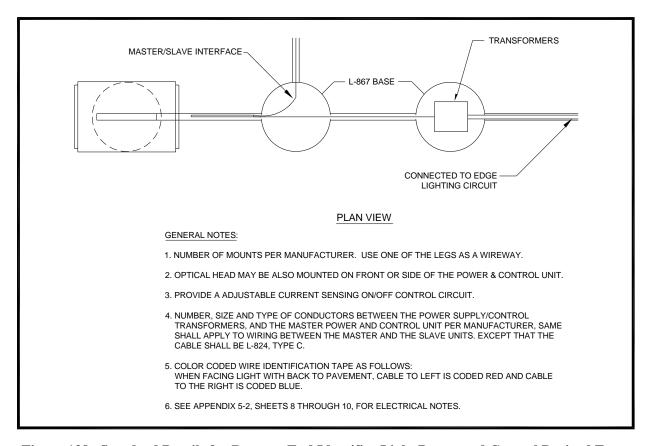
Figure 138. Standard Details for Runway End Identifier Light Power and Control Derived From Runway Circuit – Plan View
