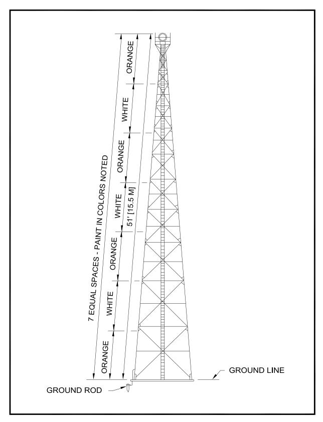
Figure 71. Typical Structural Beacon Tower
