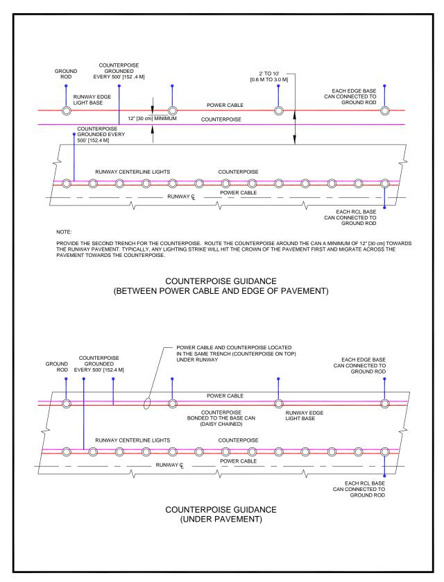
Figure 117. Typical Counterpoise and Ground Rod Connections
