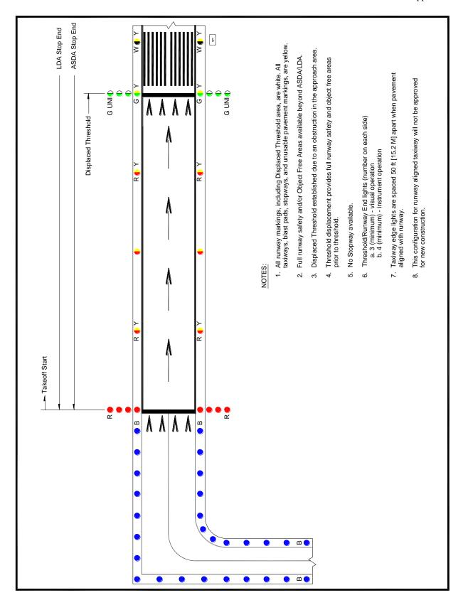
Figure 15. Lighting for Runway with End Taxiway and Displaced Threshold not Coinciding with Opposite Runway End
