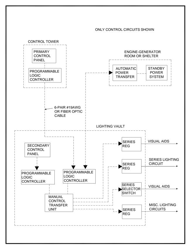
Figure 112. Typical PLC Control System Block Diagram
