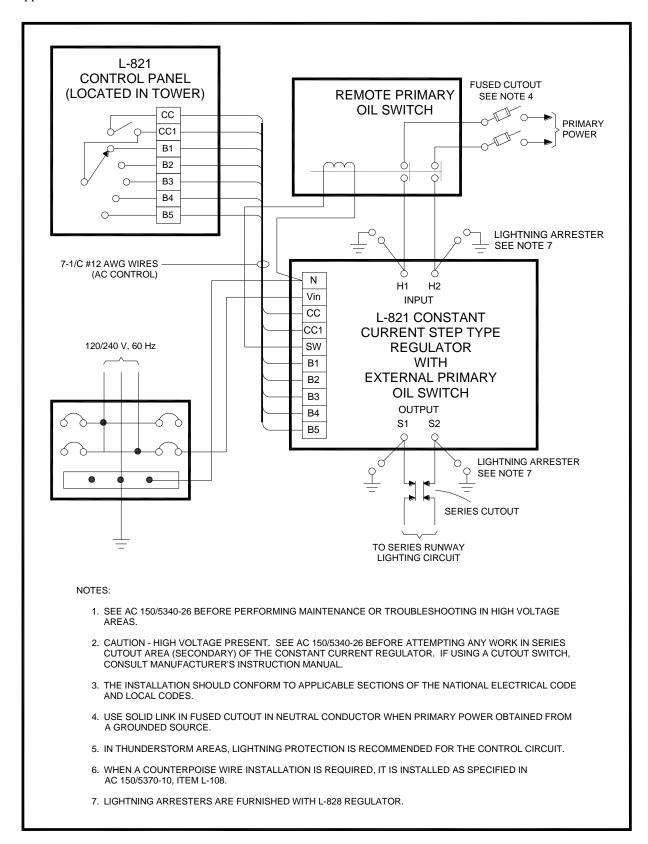
Figure 24. Typical Wiring Diagram Utilizing L-828 Step-type Regulator with External Remote Primary Oil Switch.
