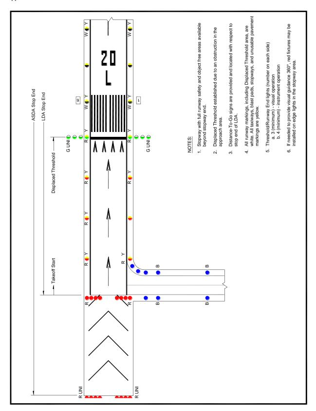
Figure 12. Lighting for Runway with Displaced Threshold and Stopway
