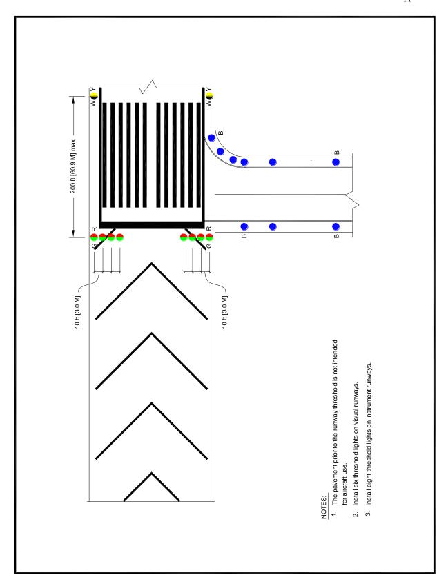
Figure 5. Runway with Blast Pad (No Traffic)
