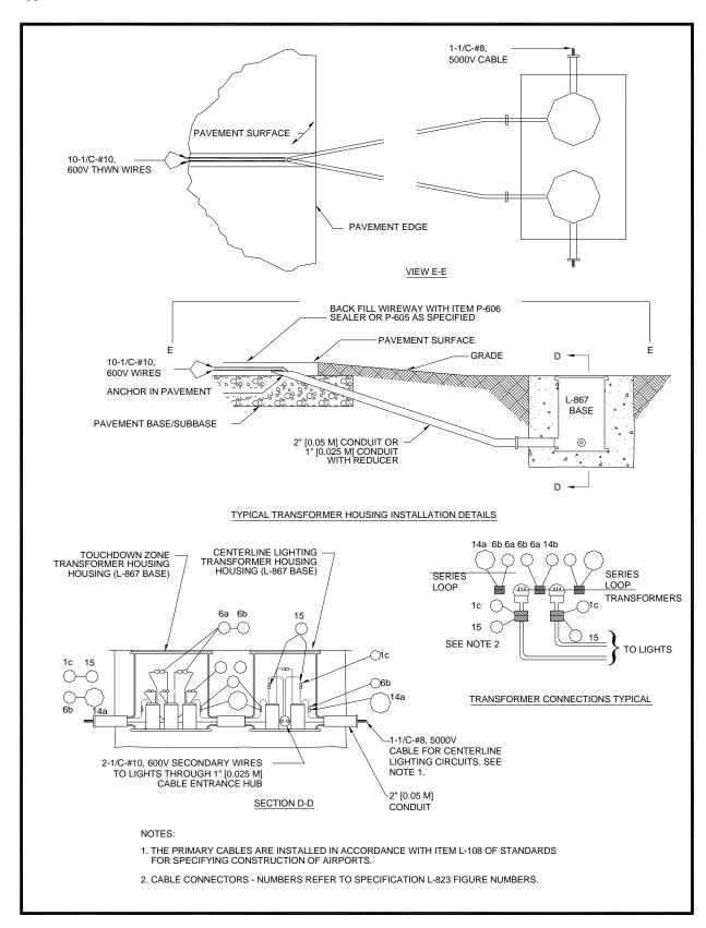
Figure 40. Transformer Housing Installation Details Inset Type Lighting Fixtures
