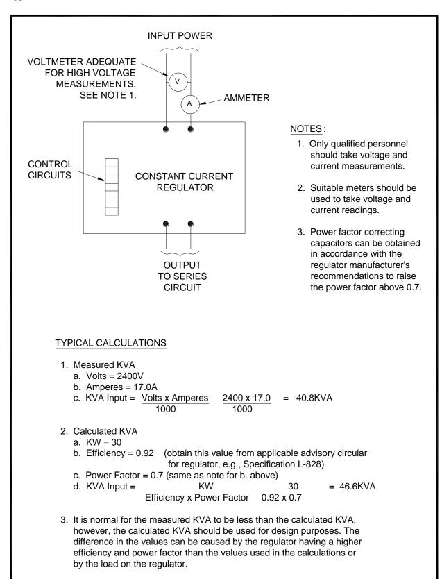
Figure 94. Typical KVA Input Requirements
