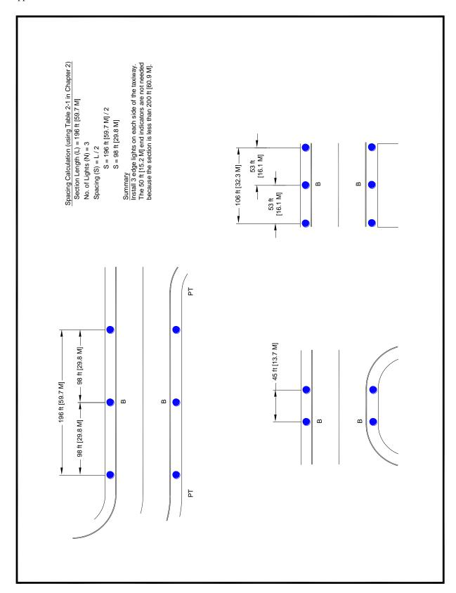
Figure 16. Typical Straight Taxiway Sections (Less Than 200 Ft. (61 m))
