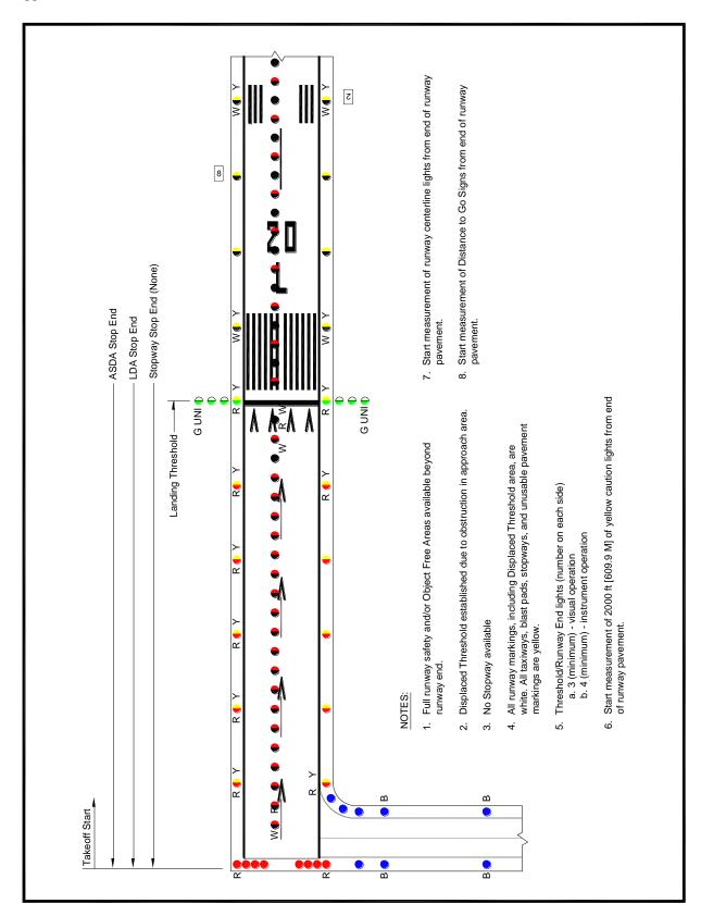
Figure 8. Lighting for Runway with Displaced Threshold
