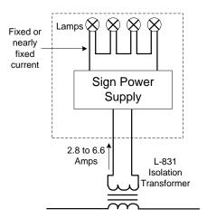
Figure 140. Controlled Output Sign Block Diagram
