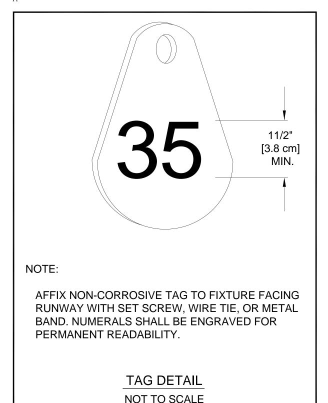
Figure 118. Identification (ID) Tag Detail
