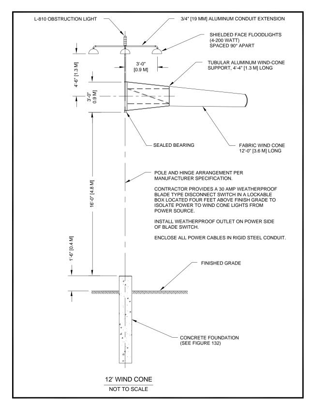
Figure 133. Standard Details for Wind Cone – 12 ft. (3.7 m) Wind Cone
