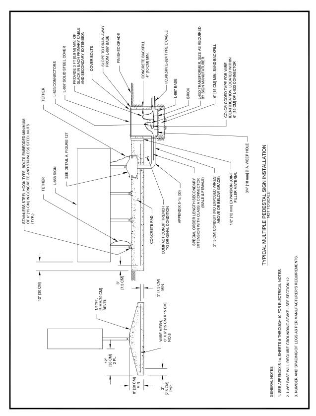
Figure 126. Standard Details for Taxiway Hold and Guidance Sign - Sign - Multiple Pedestal
