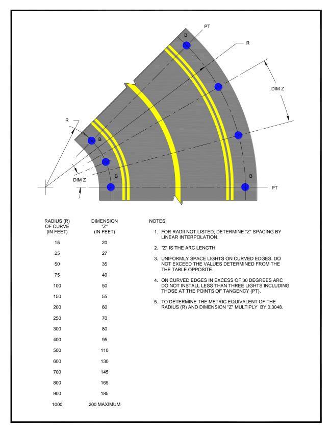
Figure 17. Spacing of Lights on Curved Taxiway Edges
