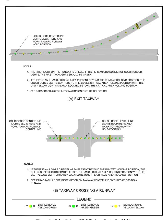
Figure 44. Color-Coding of Exit Taxiway Centerline Lights
