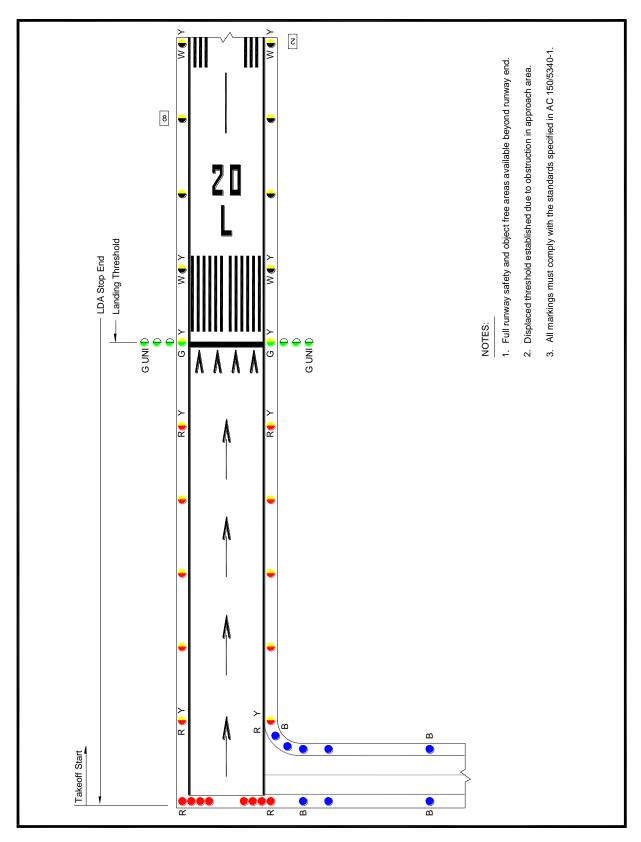
Figure 6. Lighting for Runway with Displaced Threshold
