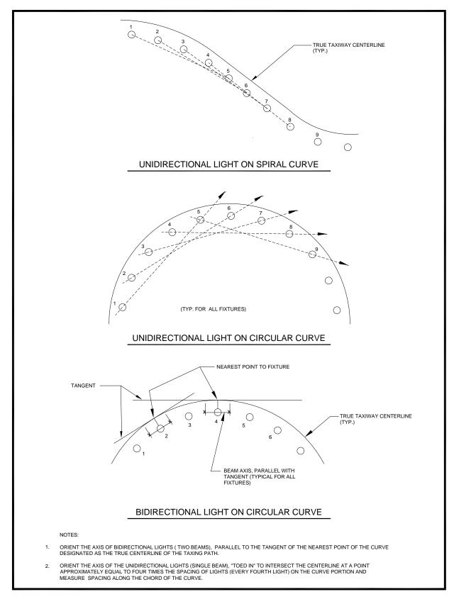
Figure 48. Taxiway Centerline Light Beam Orientation
