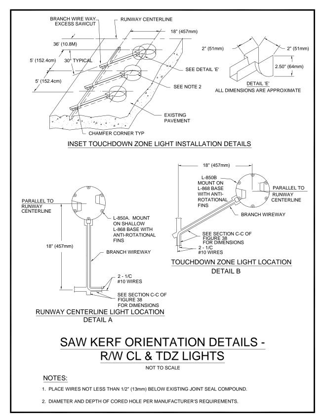
Figure 39. Saw Kerf Orientation Details – R/W Centerline and TDZ Lights
