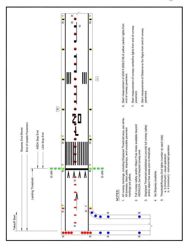
Figure 9. Lighting for Runway with Displaced Threshold/Usable Pavement
