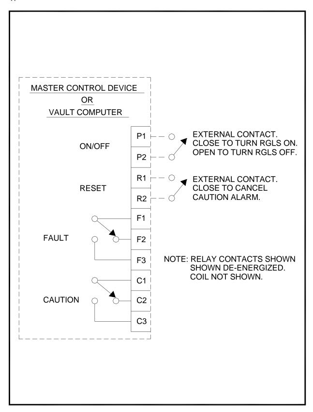
Figure 58. In-Pavement RGL Alarm Signal Connection
