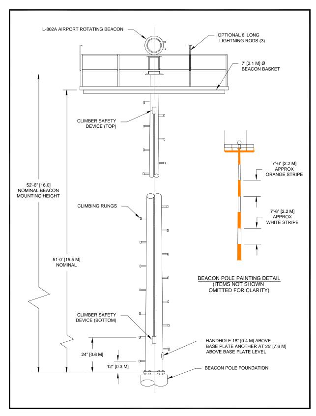
Figure 72. Typical Tubular Steel Beacon Tower
