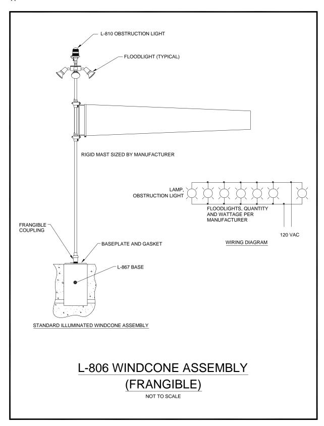
Figure 76. Externally Lighted Wind Cone Assembly (Frangible)
