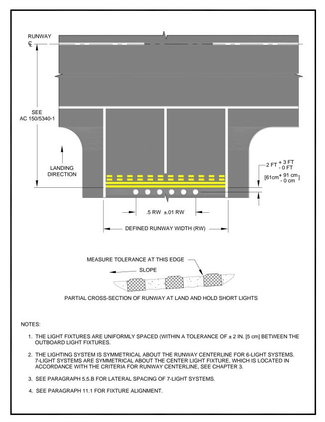
Figure 62. Typical Layout for Land and Hold Short Lights
