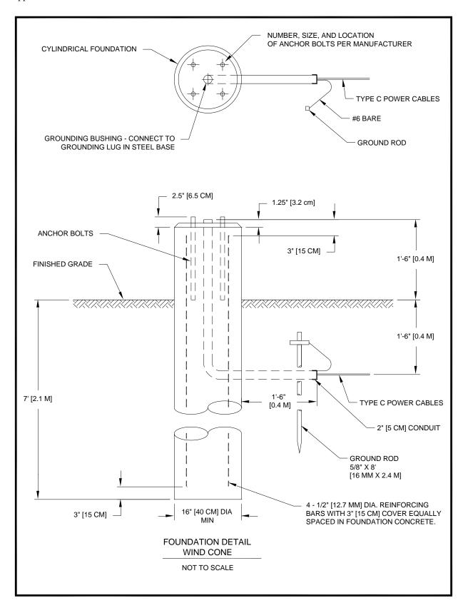
Figure 132. Standard Details for Wind Cone Foundation (L-807)
