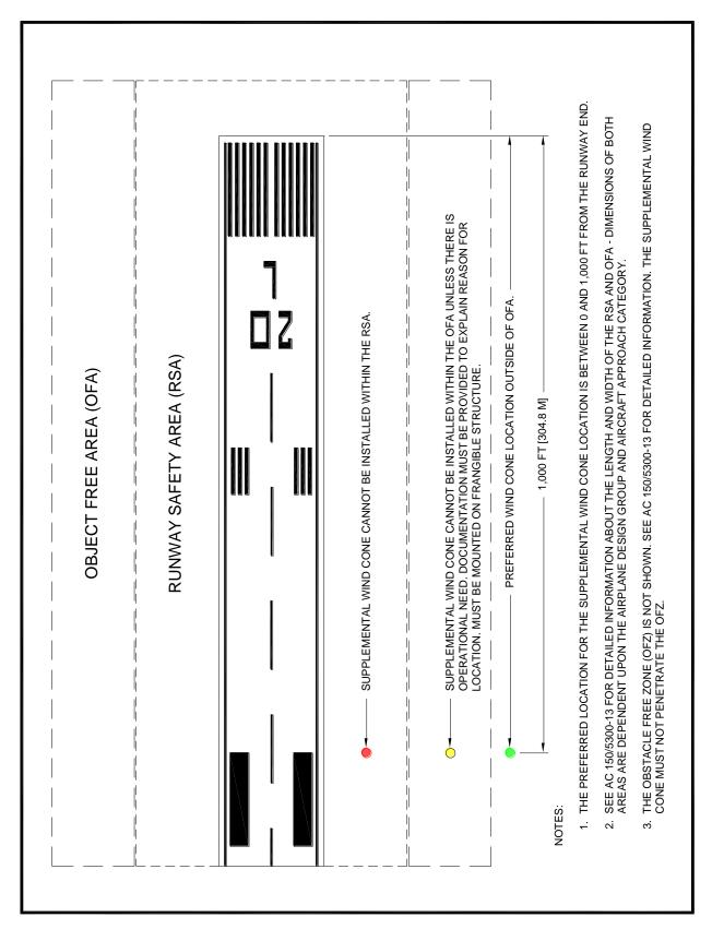
Figure 75. Typical Location of Supplemental Wind Cone
