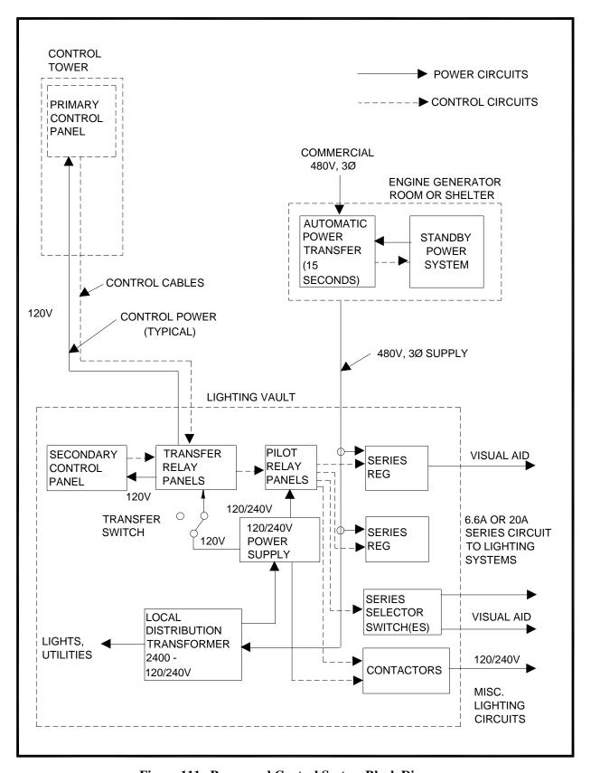
Figure 111. Power and Control System Block Diagram
