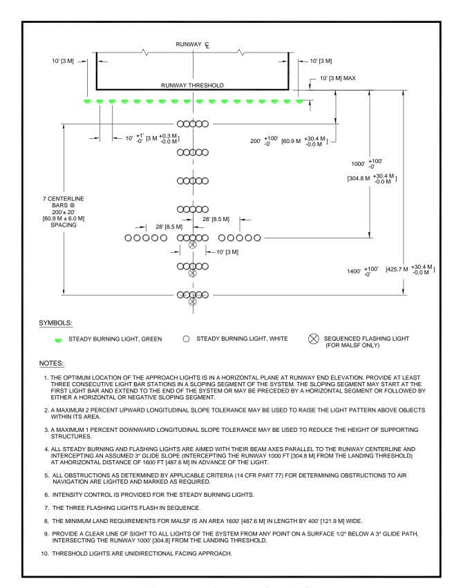
Figure 77. Typical Layout for MALSF
