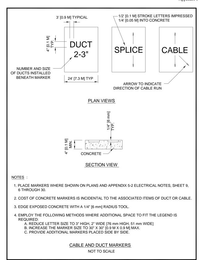
Figure 109. Cable and Duct Markers
