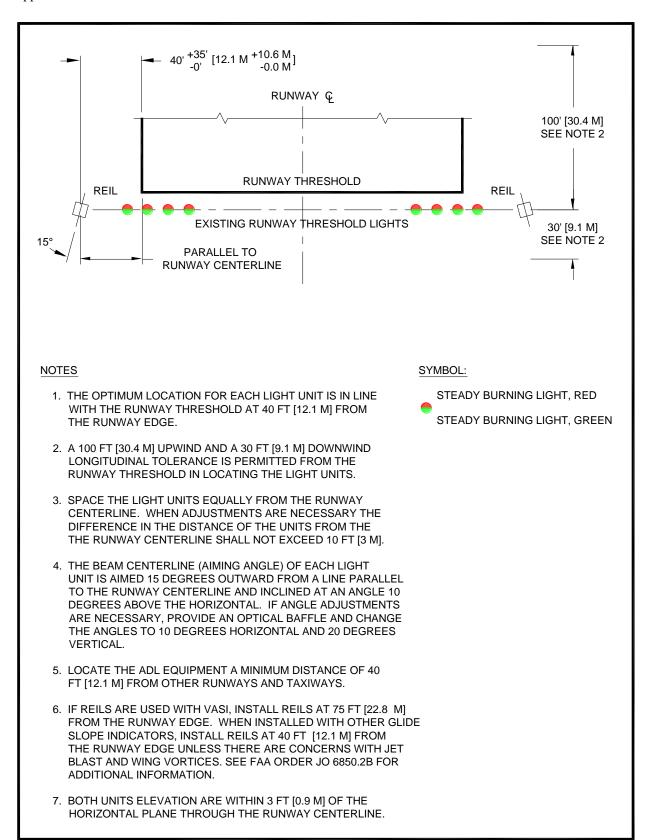
Figure 78. Typical Layout for REIL
