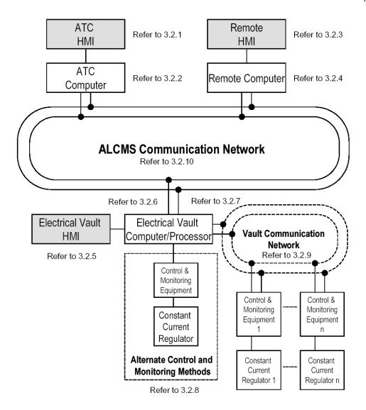
Figure 143. ALCMS Block Diagram
