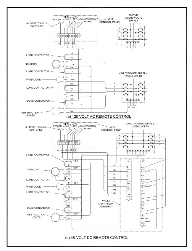
Figure 70. 120 Volt AC and 48 Volt DC Remote Control.
