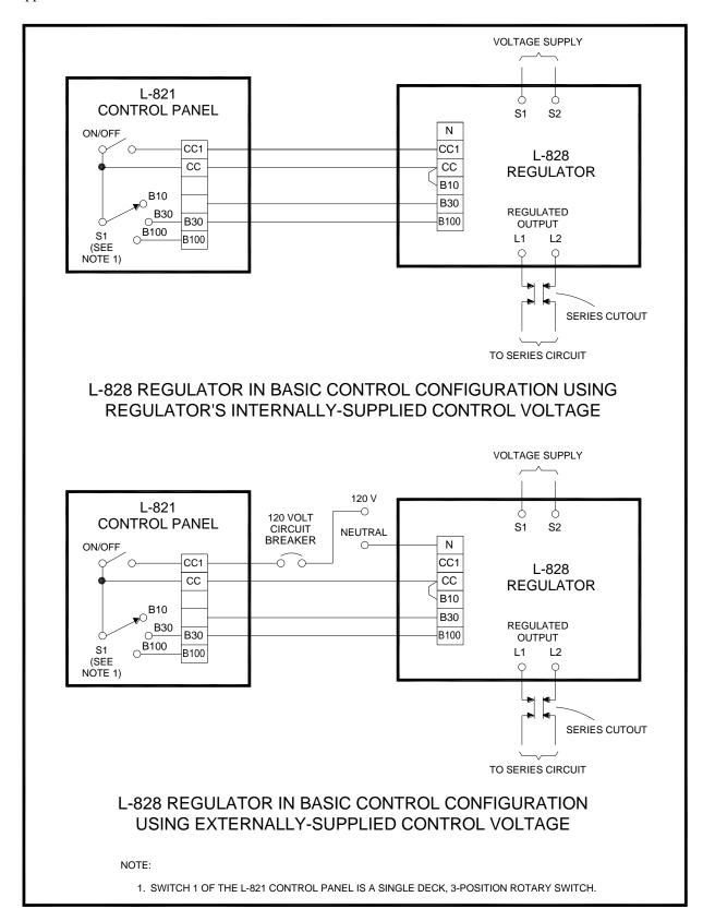
Figure 26. Typical Basic 120 Volt AC Remote Control System
