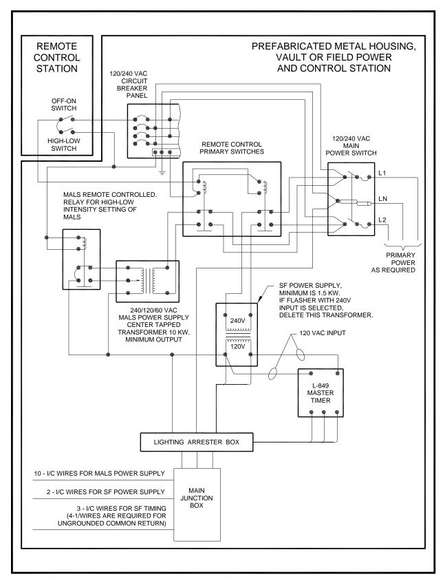
Figure 83. General Wiring Diagram for MALSF with 120 Volt AC Remote Control
