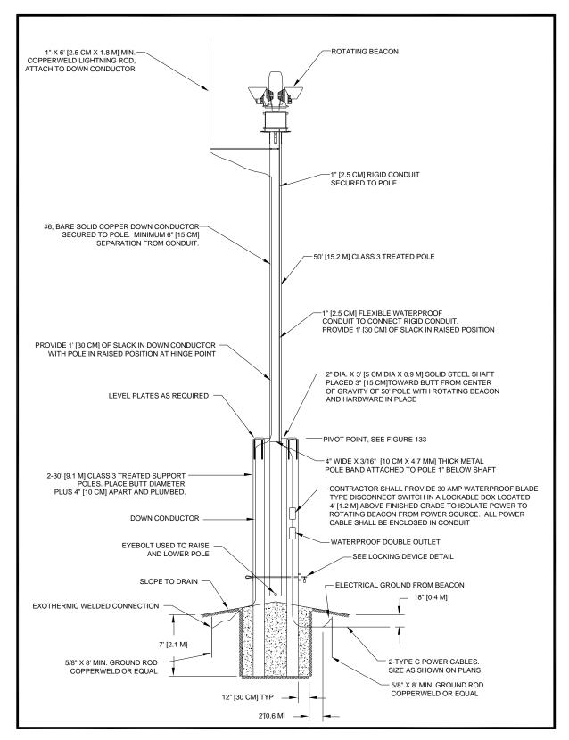
Figure 131. Standard Details for Pivoting Rotating Beacon Pole
