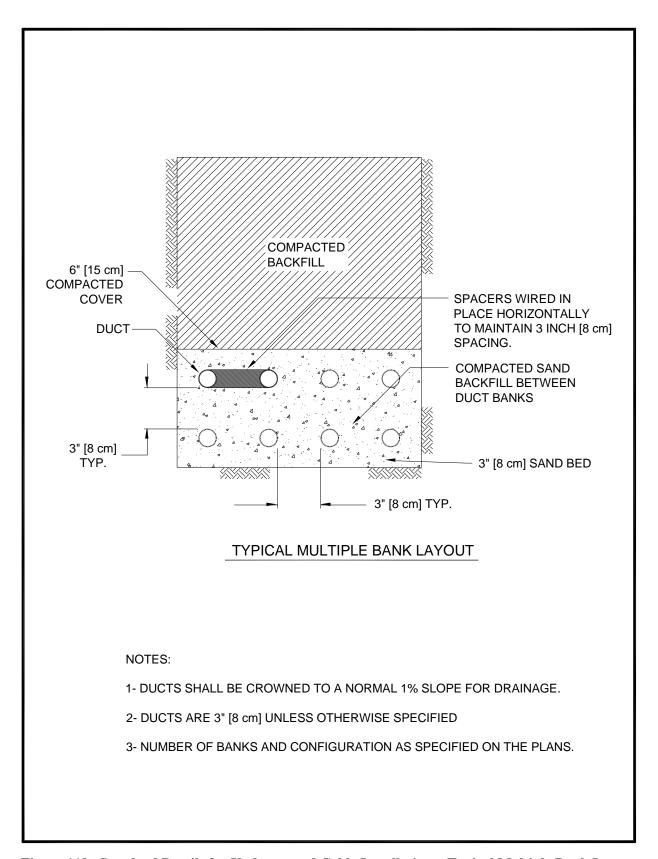
Figure 119. Standard Details for Underground Cable Installation – Typical Multiple Bank Layout
