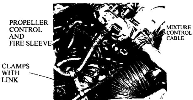
FIGURE 5. CONTROL ROUTING IN ENGINE COMPARTMENT
