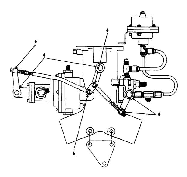
FIGURE 5. SOLID ROD ADJUSTMENT AND LUBRICATION
