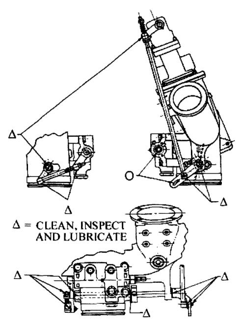
O = REFERENCE THE AIRFRAME MANUFACTURER'S INSTALLATION, CLEANING AND LUBRICATION INSTRUCTIONS
