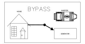
Notice that when bypassed, there is no electrical connection between the AC wiring and the inverter. This allows the inverter to be safely worked on or removed. Disconnection of the DC cabling is also required to de-energize the system.
