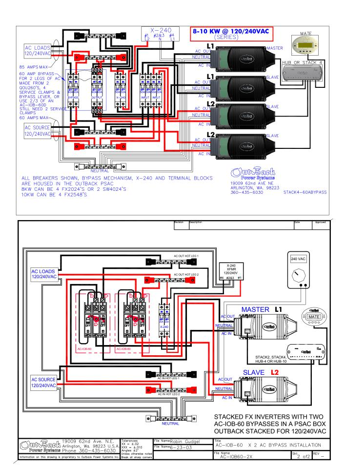
This arrangement is shown in the PSAC cabinet. (PSAC-60 + additional AC-IOB-60)
