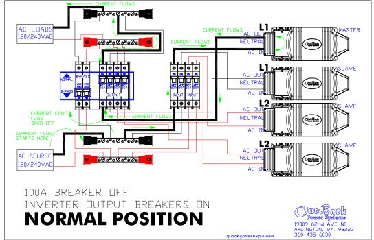
Below are examples of current flow of a quad bypass assembly. One example is shown in the normal position and the other is shown bypassed. The AC input breakers to the inverters are not mechanically tied to the bypass assembly. These inputs must be turned off separately to de-energize AC from the inverter.
