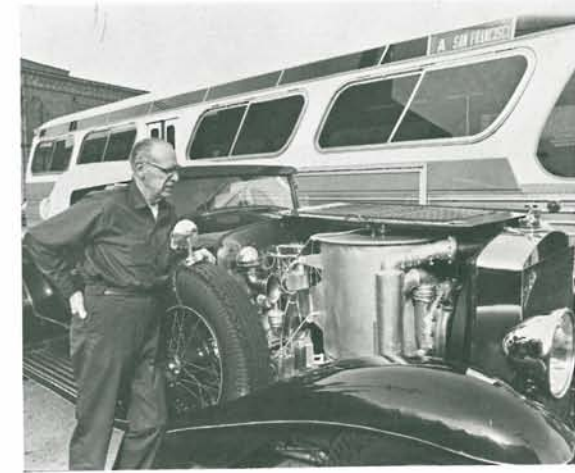
STEAM AHEAD — Modern steam plants to be installed in two District buses will be far different from that in the handsome Doble DeLuxe , built at the Doble Emeryville plant in 1924. Owner Bernard Becker of Walnut Creek, who's been "in steam" 42 years, looks at boiler under hood.
