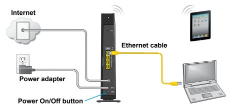
Figure 5. Modem router in a simple network
