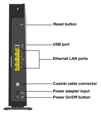
Figure 3. Modem router rear panel
