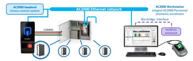
Fig. 3: Showing example of AC2000 4 door controller with optional IDEMIA Sigma biometric reader, MSO300 USB device, and AC2000 enrolment workstation
