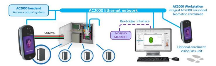
Fig. 2: Showing example of AC2000 4 door controller with optional IDEMIA VisionPass facial biometric reader and AC2000 enrolment workstation.
