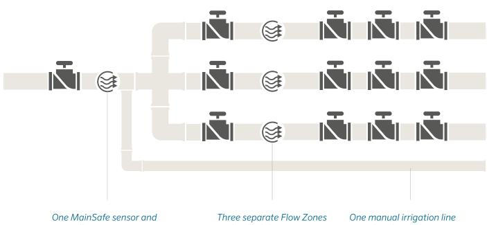
normally open master valve monitors the entire water source, including total monthly usage. Three separate Flow Zones each schedule stations on to safe, optimum target flow rates for the specific diameter of mainline pipe. One manual irrigation line provides always-on irrigation on demand, but is still monitored by the upstream MainSafe master.
