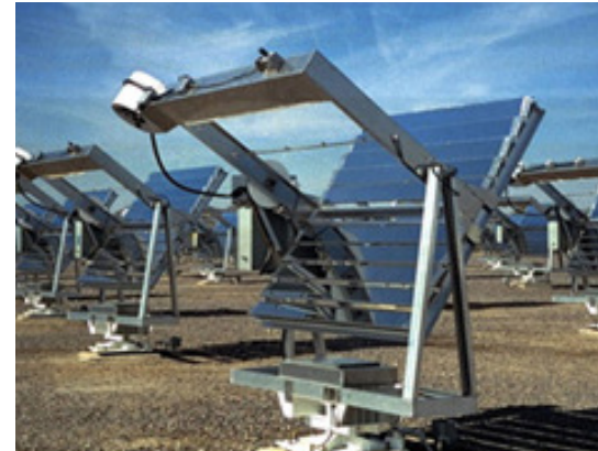
Q-Trac Natural Sunlight Concentrator Testing photo provided by Q-Lab, www.q-lab.com
