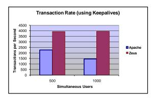
Using Keepalives with Zeus Traffic Manager adds a further performance boost. Note that the Apache server was the bottleneck in all these tests, running at between 90% and 100% CPU utilization. The Zeus Traffic Manager had ample spare capacity to load-balance traffic across a number of Apache servers.
