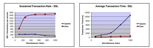
During the tests, many of the connections to the Apache server failed due to timeouts. When Zeus Traffic Manager was used to decrypt the connections, no failures were observed:
