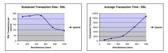
Then Zeus Traffic Manager was used to transparently decrypt SSL traffic on behalf of the Apache server, so that it processed unencrypted traffic only.
