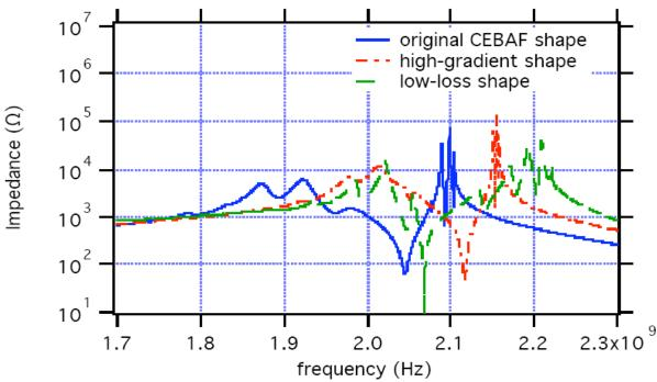
7-cells, OC, HG, LL shapes,  $TE_{111}/TM_{110}$  dipole, beam-pipe damping
