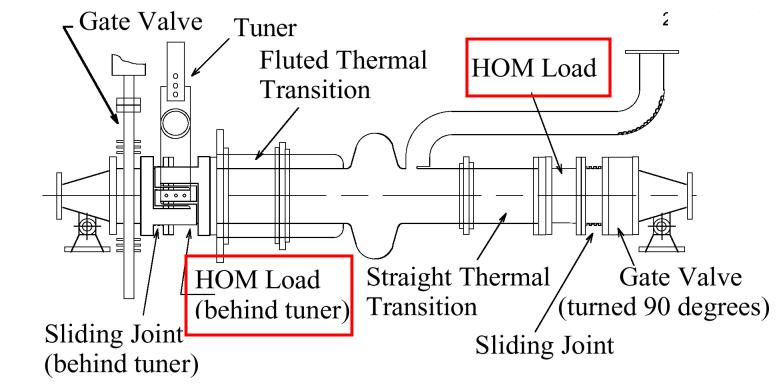
$\succ$  Flute beam pipe  $\Rightarrow$  guide out the first two defecting modes.
