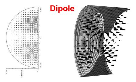
Figure 6: One mid-cell of a TESLA cavity. The electric field of the 1.79 GHz  $\pi$ -mode of the first dipole passband is shown. The left graph shows the electric field in a plane perpendicular to the cavity axis.
