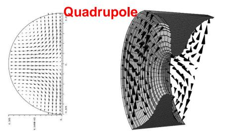
Figure 7: One mid-cell of a TESLA cavity. The electric field of the 2.32 GHz  $\pi$ -mode of the first quadrupole passband is shown. The left graph shows the electric field in a plane perpendicular to the cavity axis.
