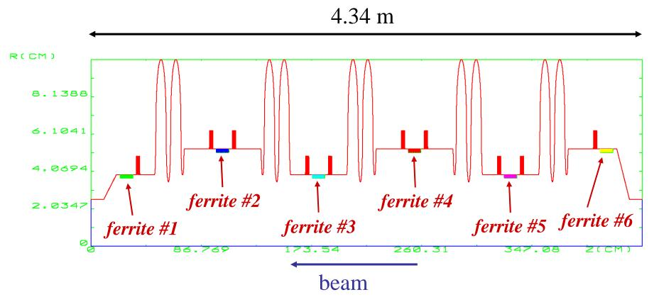
HOM damping concept: Make all TM monopole and all dipole modes propagating by increasing the beam tube diameter (as in CESR).
