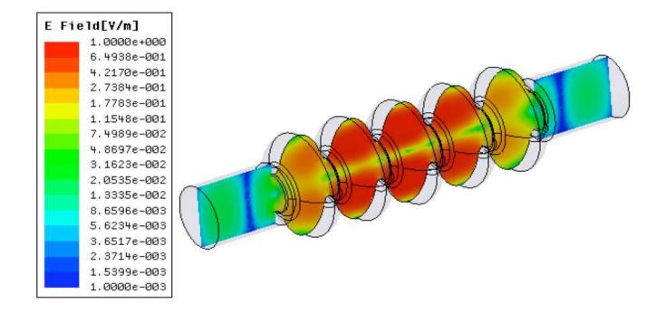
HFSS 3D complex Eigenvalue solution, 5-cell cavity with enlarged beam-pipes.
