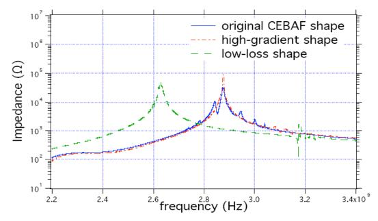
TM011 band, OC, HG, LL shapes, 7-cells, beam-pipe damping
