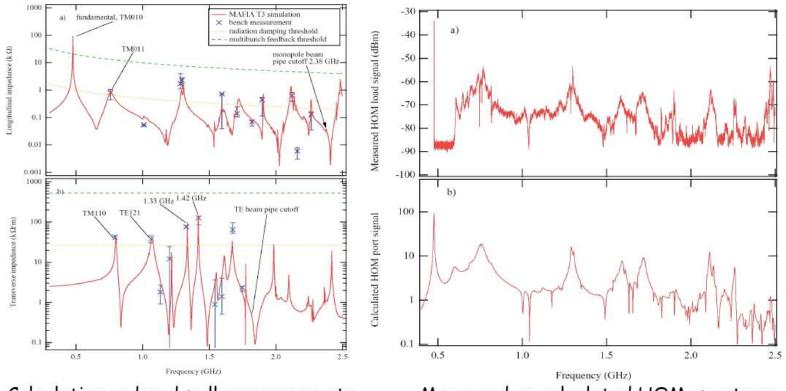
Calculation vs bead-pull measurements.
