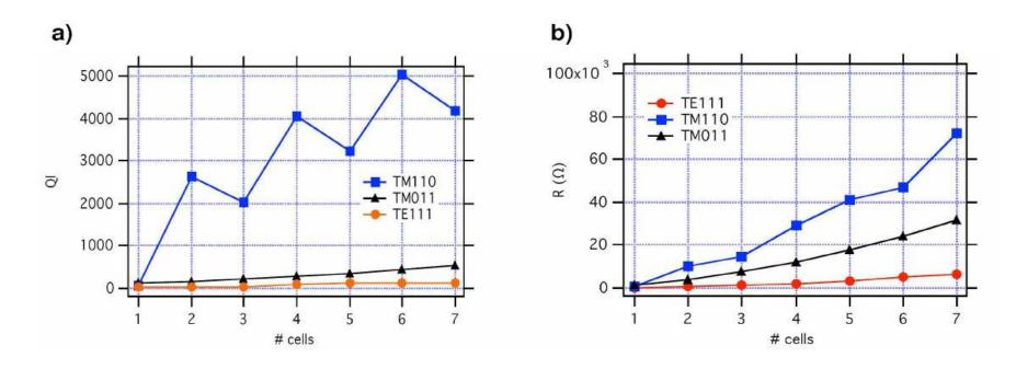
Fig. 11. Impact of number of cavity cells on HOM impedance (TM011, TE111 and TM110 passband modes with beam pipe damping). a) Loaded Q vs. number of cells.b) Impedance vs. number of cells (dipoles at 25 mm transverse offset). Courtesy of B. Rimmer.
