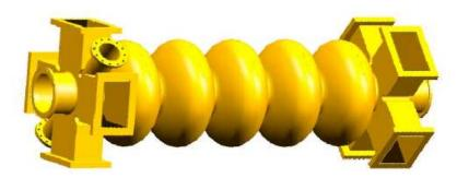
5-cell waveguide damped cavity
