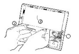
Figure 2. Removing the PCB
