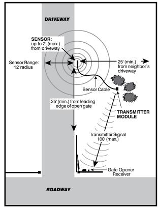
Sensor Range distance is approximate and will vary due to outside interference, vehicle mass, speed, etc.
