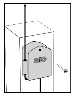
Step 3: Connect the RED and BLACK wires from the Receiver to the power supply (see illustration, page 5).
