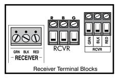
**Step 1:** The RB709U-NB will replace the gate opener receiver; disconnect the gate opener receiver's RED, BLACK, and GREEN wires from the receiver terminals on the gate opener control board.
