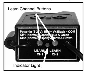
Note: You will have to use a small screwdriver or a pen to depress the LEARN CH buttons on the receiver.
