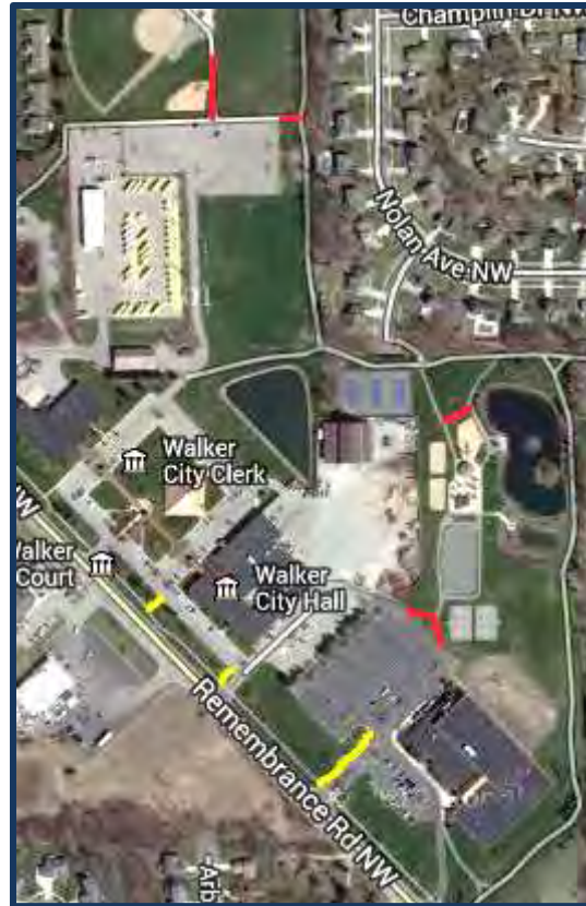
Figure 3: Paths with a slope exceeding 1:20. Original image taken from Google Maps
