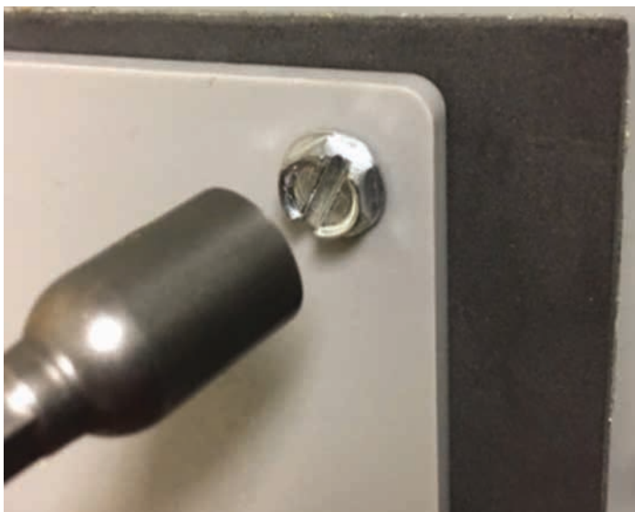
Use to tighten or loosen WMEP plate screws.
