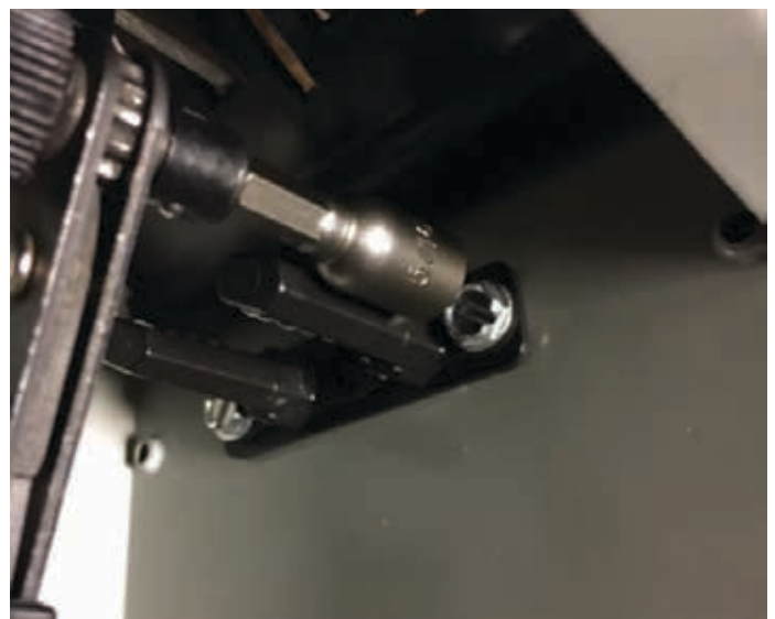
Use to remove Quick Bolt™ assembly on invertible tap boxes.
