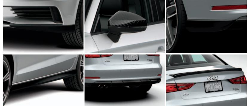
A3 body kit—Front spoiler with blade insert This styling component creates a lowered appearance. Blade is primed for painting.
