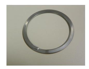
Lock ring with evidence of tampering. Note the multiple impact points similar to those made by a flathead screwdriver. In addition, the overlapping sections of the lock ring are no longer flush
