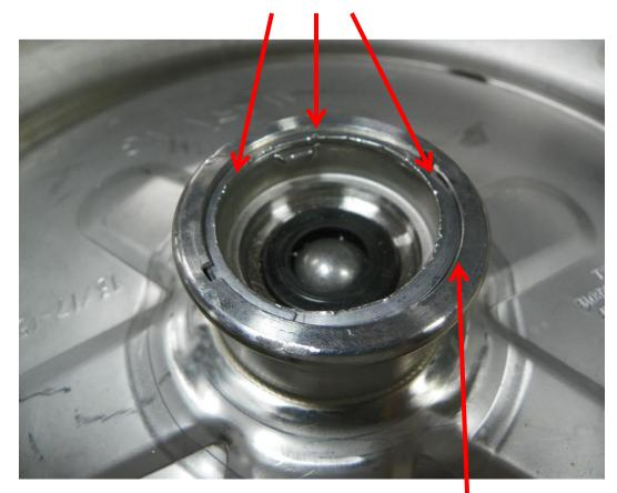
Bent ear prevents the lock ring from fitting into lock ring channel
