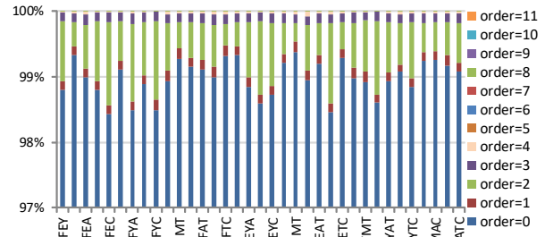
Figure 7: The distribution of allocation orders. The corresponding allocation size equals to 2^{order} [21].
