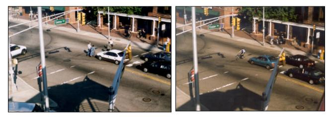
Pictures 2.3-5 and 6: A typical conflict – the motorist pulls into the crosswalk because the far side signal allows him/ her to do so – the pedestrians/ cyclist are forced to cross in or near the path of turning vehicles. New Brunswick, NJ.
