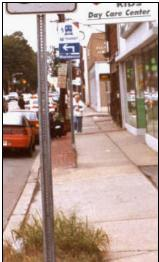
Picture 4-2: Typical sidewalk condition – minimum width and poorly maintained. Maplewood, NJ.
