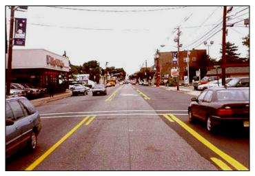
Picture 4-1: Typical crosswalk condition – striped but hardly visible. Maplewood, NJ.
