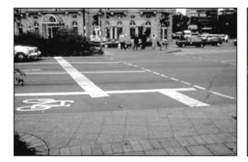
Picture 3.6-1: Recessed stop line also allows cyclists to get a head start before motor vehicles, thus making them more visible to motorists.
