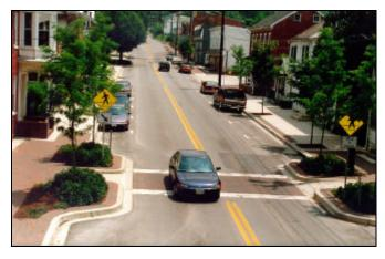
Picture 3.1-2: Mid-block crossing with curb extension to reduce crossing distance for pedestrians. Westminster, MD.
