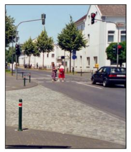
Picture 2.3-7: Near side signal only – motorists are naturally forced to stop at stop line because otherwise he/ she would not be able to see the signal. Germany.
