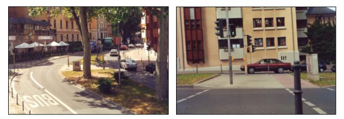
Picture 3.4-1: A crosswalk, nice wide median and two-phase push-button signal with almost immediate response ensures a safe and convenient crossing for pedestrians (and cyclists). Germany.
