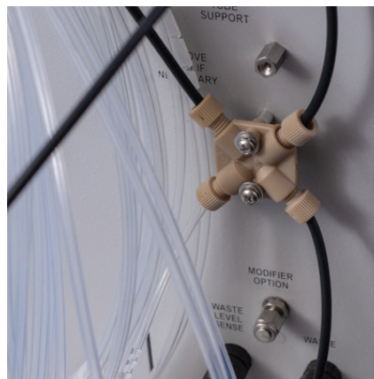
Figure 2-21 AutoSampler waste connection point on ACCQPrep
