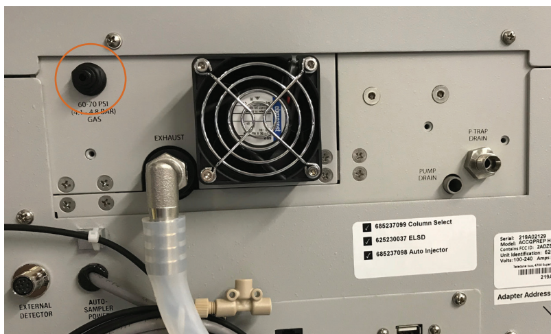
Figure 2-9 Location of ELSD gas port (Nitrogen input line circled)
