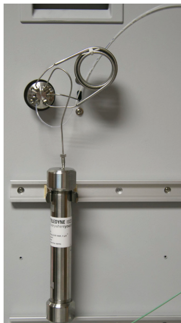
Figure 2-34 Column with inlet and outlet lines connected
