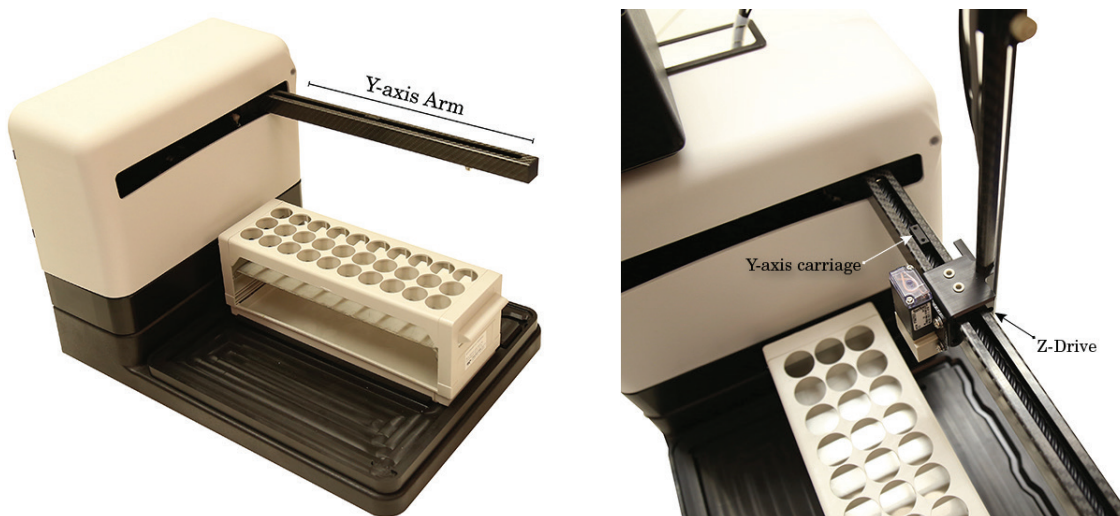
Figure 2-16 Z-Drive mounted on the Y-axis carriage
