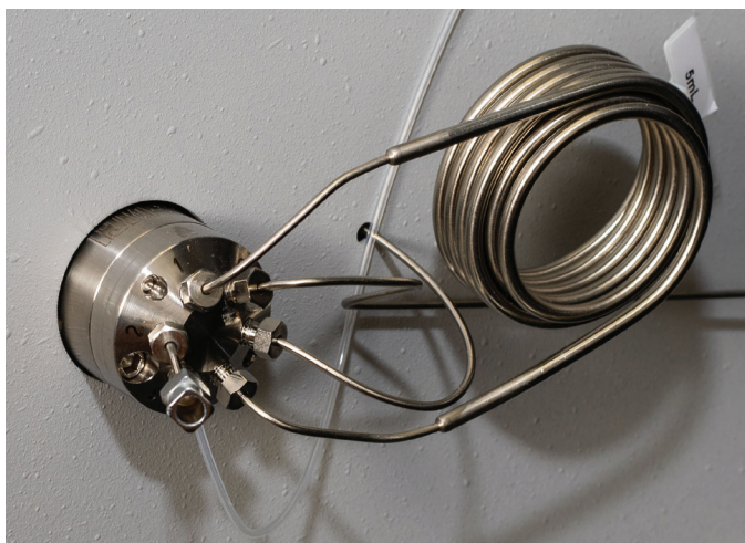
Figure 2-14 ACCQPrep with Manual Injection Luer Port installed
