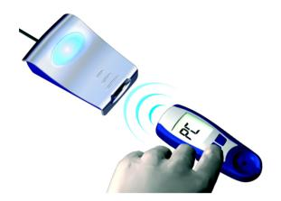
The Accu-Chek Active meter has an infrared port for data transfer. In order to read data from these meters, proceed as follows:
