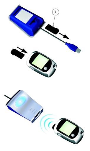
The Accu-Chek Comfort meters use the contacts for the coding chip as an interface for data transfer. In order to read data from these meters, proceed as follows:
