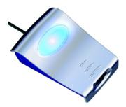
Plug the USB connector of the Accu-Chek Smart Pix device into a free USB socket on your computer. When you do this it does not matter whether the computer is switched on or off. The Accu-Chek Smart Pix device is also supplied with electricity via this connection so it does not require any batteries or power pack.
