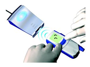
The Accu-Chek Compact/Integra meter has a built-in infrared port for data transfer. In order to read data from these meters, proceed as follows:
