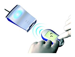
The Accu-Chek Aviva meter has a built-in infrared port for data transfer. In order to read data from these meters, proceed as follows:
