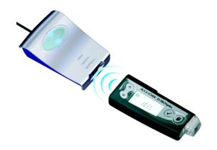
The insulin pump Accu-Chek D-TRONplus (Disetronic D-TRONplus) has a built-in infrared port for data transfer. In order to read data from these meters, proceed as follows:
