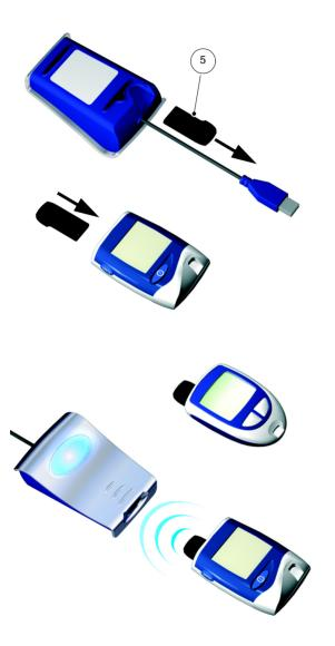
The Accu-Chek Sensor/Advantage meters use the contacts for the coding chip as an interface for data transfer. In order to read data from these meters, proceed as follows:
