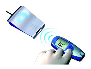
The Accu-Chek Go meter has a built-in infrared port for data transfer. In order to read data from these meters, proceed as follows:
