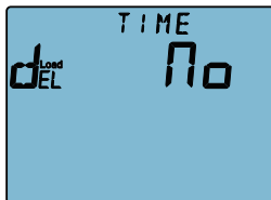
Fig.3-53 Clear load running time setting
