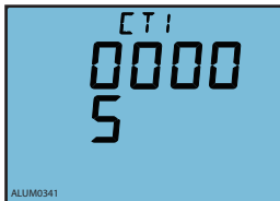
Fig.3-44 CT primary side ratio setting
