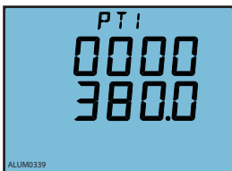
Fig.3-42 PT primary side ratio setting
