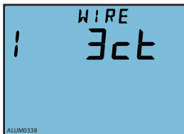
Fig.3-41 Current input wiring setting
