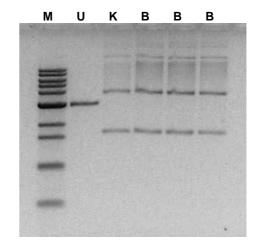
Figure 3. Re-ligation of gel-purified DNA. Gel-purified DNA was ligated by T4 DNA ligase after purification using Bioneer's AccuPrep<sup>®</sup> Gel Purification Kit (B) and competitor's kit (K).
