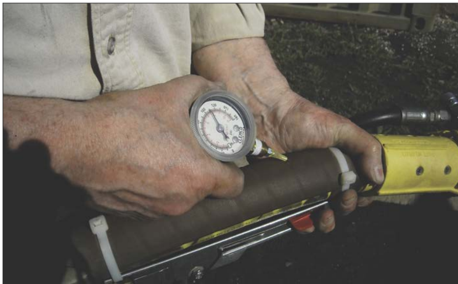
Fig. 2: Needle pressure gauge used to check pressure at the nozzle.
