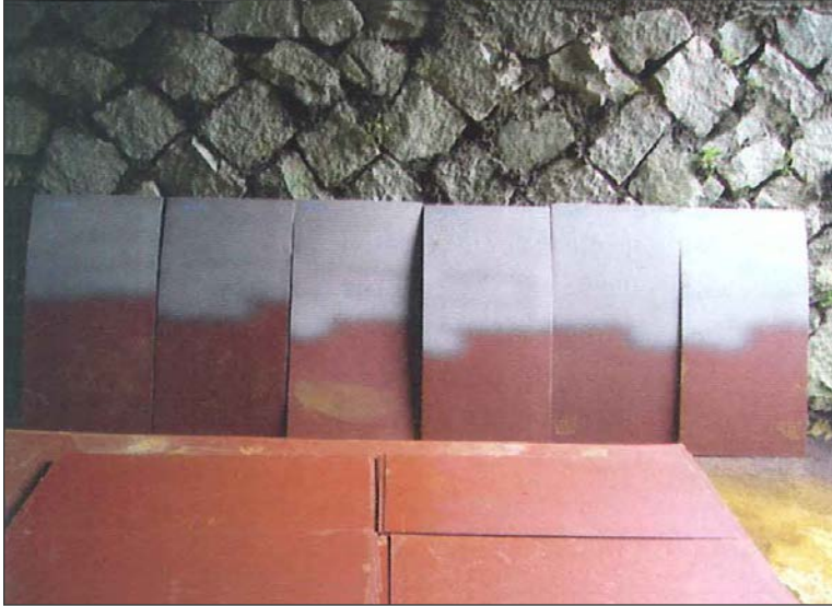
Fig. 2: Appearance of specimens after blast cleaning test
