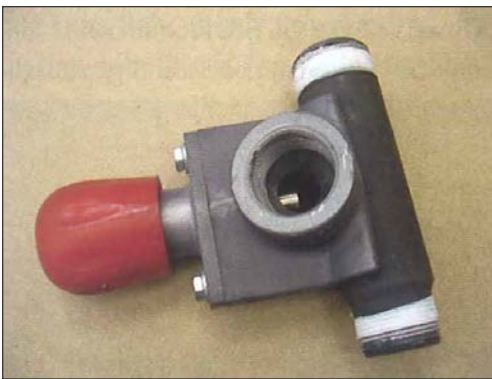
Fig. 6: Newer type of abrasive metering valve that allows more precision than spring type
