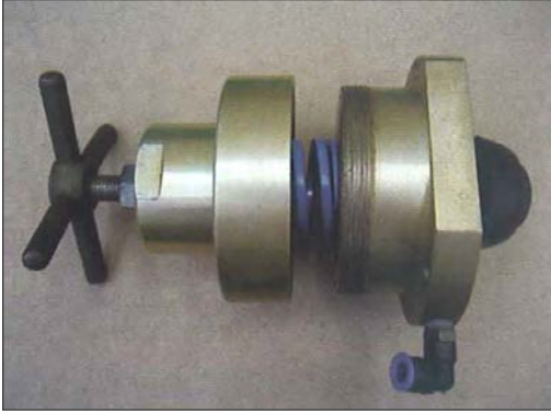
Fig. 5: Older spring-type of abrasive metering valve still used in some shipyards
