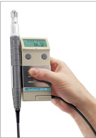
Fig. 2: A handheld digital gage for measuring air temperature, surface temperature, and relative humidity. It uses the values to calculate dew point and the difference between the dew point and the surface temperature. Courtesy of Defelsko
