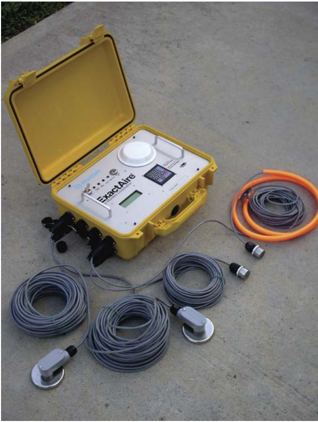
Fig. 1: Monitor with 24-hour uplink to internet with secure access allows surface temperature, ambient conditions, and dew point spreads to be checked from a remote location. Courtesy of Munters Moisture Control Services
