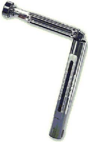
Fig. 3: A sling psychrometer (above) along with a surface temperature gage and psychrometric charts can be used to determine dew point and relative humidity. Courtesy of Bacharach
