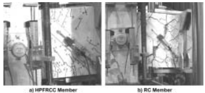
Fig. 13—Damage in HPFRCC and RC flexural members at 4.0% drift.
