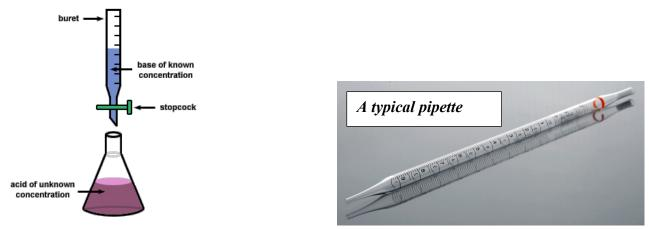
The "standard" solution, of known concentration is typically added to the buret. The solution of unknown concentration is typically added to the Erlenmeyer ("conical") flask. A specific volume is added to the flask (usually 10.0 or 25.0 mL) using a **pipette** which also measures volumes very precisely. The sample size (in mL) of the unknown is called an "aliquot."
