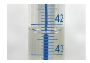
This volume information would be written in a data table like this:INITIAL BURET READING: $18.50 \pm 0.05 \text{ mL}$ FINAL BURET READING: $42.30 \pm 0.05 \text{ mL}$ TOTAL VOLUME OF NaOH used in the Titraion: $V_f - V_i = 42.30 - 18.50 = 23.80 \text{ ml}$
