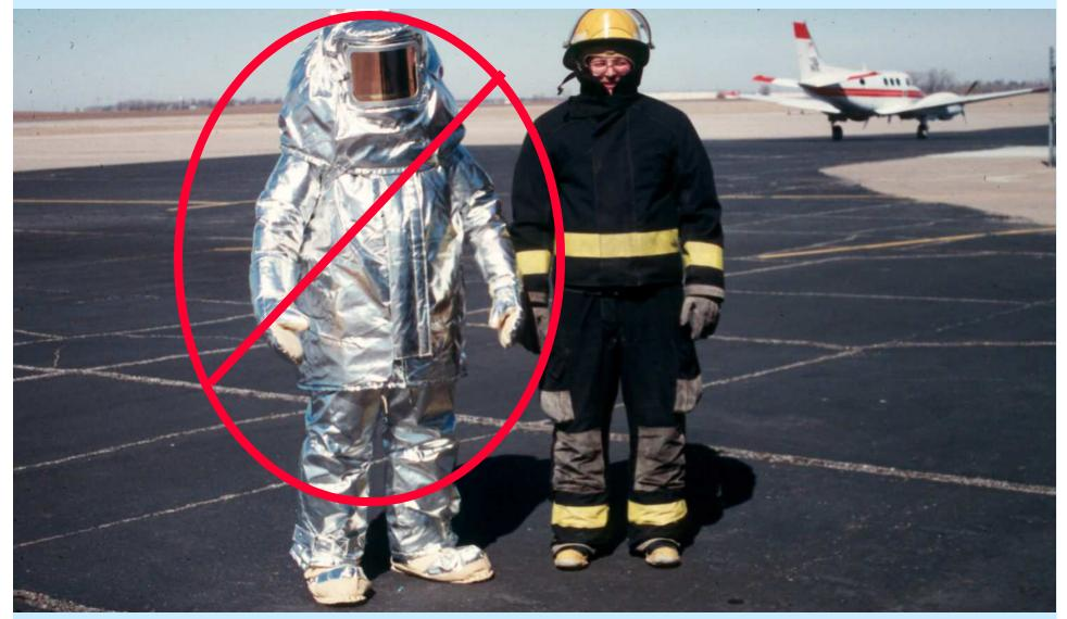
The Aluminized Fyrepel Model 700 suit on the left is an industrial type suit and is not designed for firefighting 24
