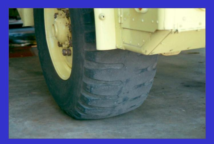
Check the condition of tires - worn tires provide poor traction in muddy off-pavement conditions
