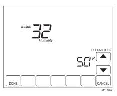
2. Use Up and Down arrow keys, located to the right of the dehumidifier setpoint, to set your desired humidity level (select models) for dehumidification in the summer.
