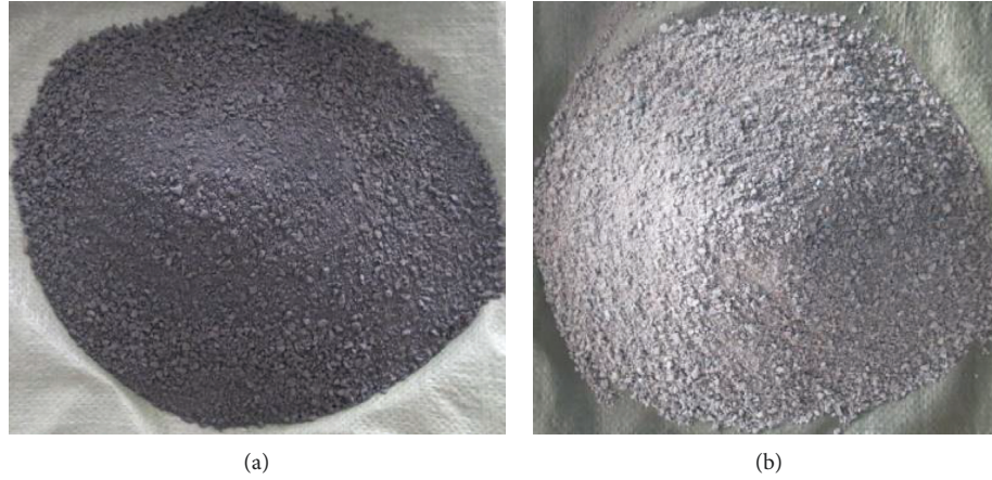
FIGURE 2: Coal gangue and wasted concrete fine aggregate. (a) Coal gangue. (b) Wasted concrete.
