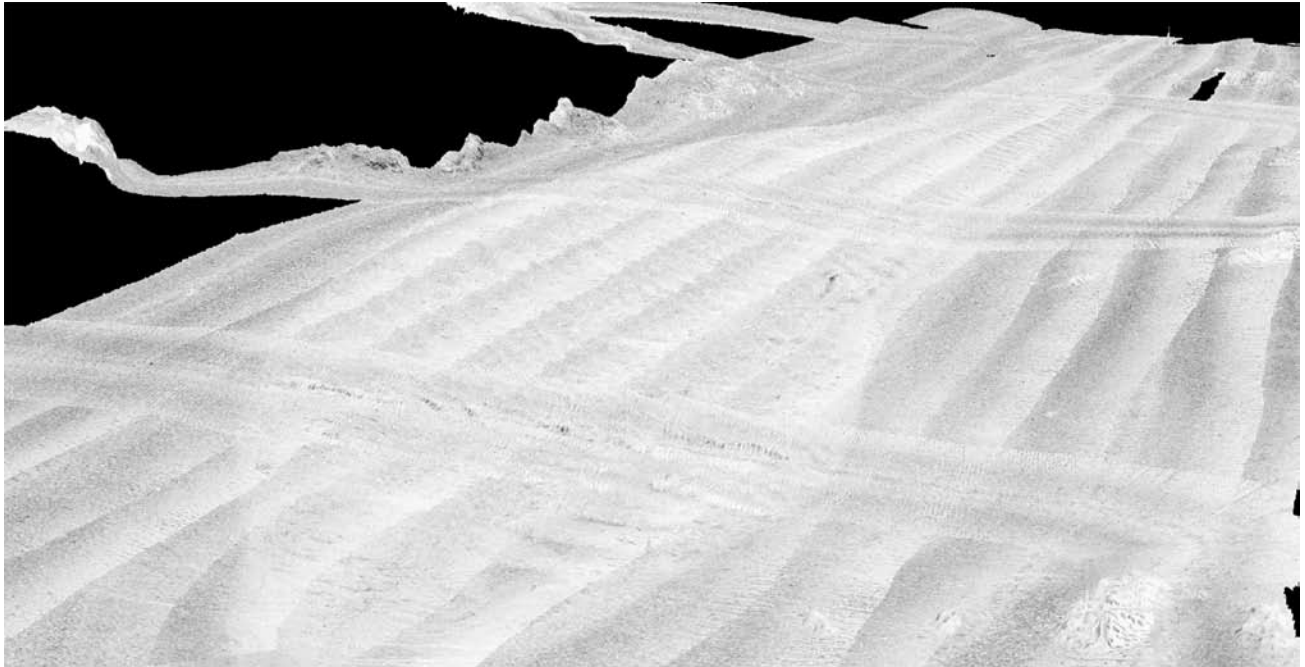
Figure 12. Direct mosaic of backscatter from multibeam sonar receiver output.
