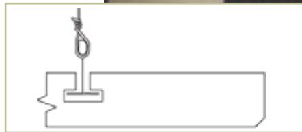
◀ Cloud with Tee and Hanger Wire
