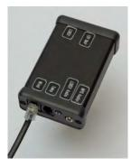
Figure 4.9: Weather connection into the interface box
