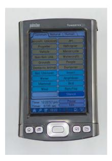
Figure 3.7: Palm Tungsten T5 running NPS Soundscpe software
