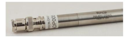
(c) Dummy mic connected
