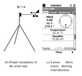
Figure 4.12: Orienting the wind vane
