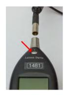
Figure 4.7: Microphone cable connection to the LD831
