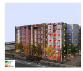
Three-dimensional noise model provides an accurate visual "heat map" of project noise levels
