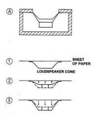
Figure 1.1. Cross-section of a loudspeaker box seen from the side, and stages 1 to 3 described in the text. The arrows mark the position of the loudspeaker membrane in relation to its equilibrium and the varying air pressure (the sound pressure) acting on the paper sheet, respectively.
