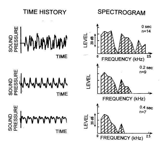
Figure 1.9. Time history (left plots) and spectra (right plots) of a guitar tone immediately after attack, 0.2, and 0.4 seconds later.
