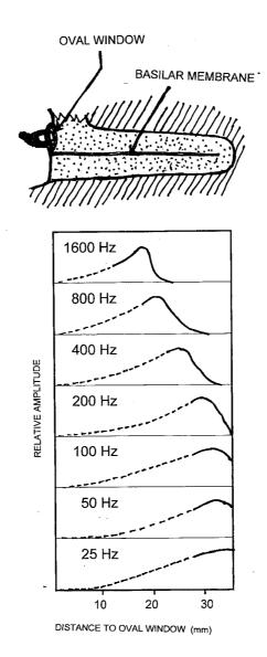
Figure 1.13. a) Sketch of the function of the outer ear (upmost picture). The cochlea has the shape of a spiral with 2 and 3/4 turns, but has been drawn straight to give a clearer picture (after Hadding and Petersson). b) The
