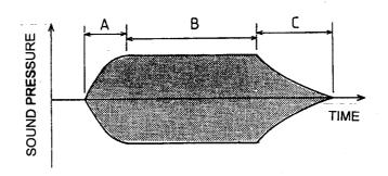
Figure 1.5. Time history of a tone in principle: A the starting transient, B the constant (more or less) part, and C the ending transient (the oscillations are generally to close to be drawn, and are marked here by the shade).
