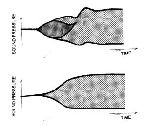
Figure 1.7. Time histories (shaded oscillograms) of starting transients of two pipe organ tones, the same pipe differently adjusted. In the upper frame the second partial dominates initially (dark area) the time history, in the lower frame the fundamental (the lowest partial) just grows (after Sundberg 1966).
