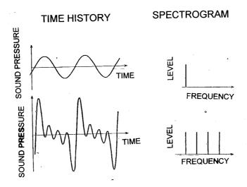
Figure 1.4. Time histories (left) and spectra (right) for a) a simple tone (upper plots), and b) a more real tone (lower plots) with four equally strong partials.
