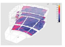
Interior computer model of a 2,100 seat multiuse concert hall, used to develop recommendations for acoustical treatment and room shaping.
