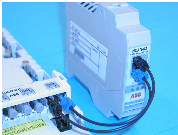
Figure 4 - 14 NCAN-02 fieldbus module installed on CH0 of RDCO-01C option.
