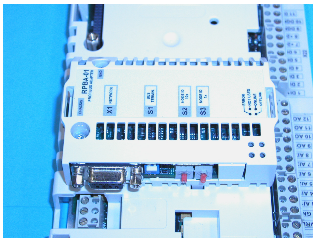
Figure 4 - 15 RPBA-01 fieldbus module installed in Slot 1 on to the RMIO board.
