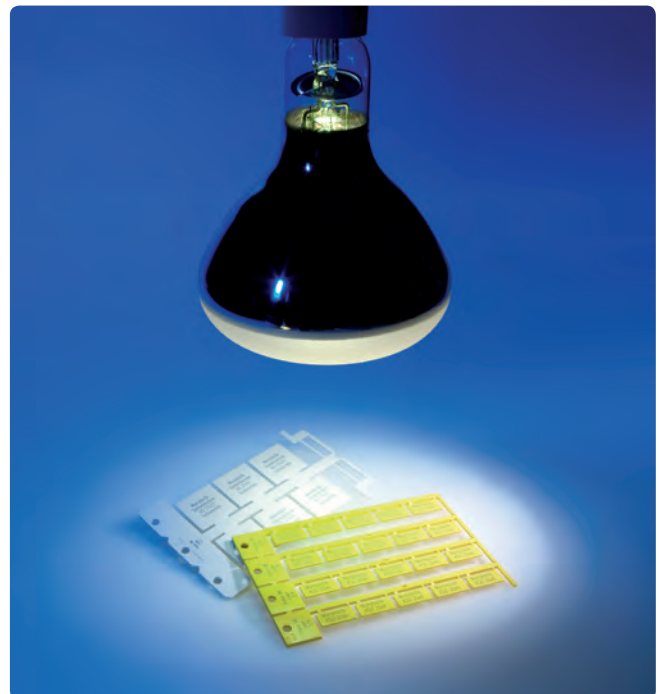
UV light stability test
