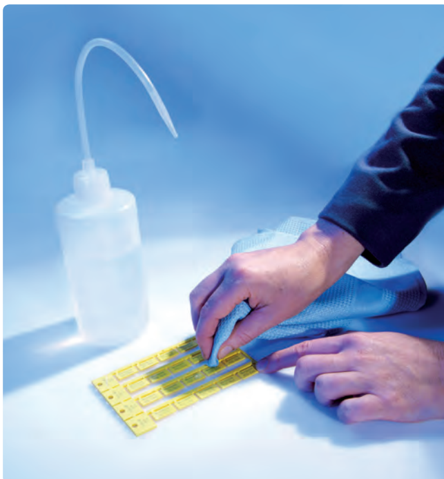
Smudge resistance test
