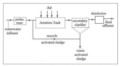
Extended Aeration Activated Sludge Wastewater Treatment Process
