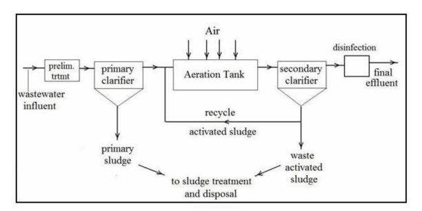
Activated Sludge Wastewater Treatment Flow Diagram
