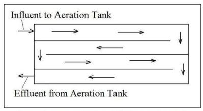
Serpentine Pattern Activated Sludge Aeration Tank
