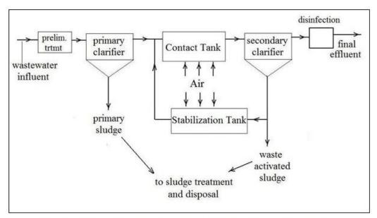
Contact Stabilization Activated Sludge Flow Diagram
