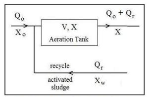
Aeration Tank Material Balance Diagram
