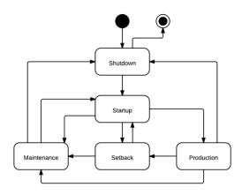
Figure 4 - UML State Diagram of Paint System Operating States
