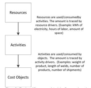
Figure 2 - Tracing of Resource and Activity Consumption using Resource and Activity Drivers [1]
