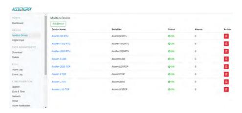
A device that is successfully connected and communicating with the gateway will have a green 'ON' mark under the status column. Whiles a device that is offline will display a red 'OFF' warning symbol.
