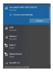
Once connected to the gateways wireless network, open up an internet browser and enter in the IP address **192.168.100.1**. The following login screen will be prompted.
