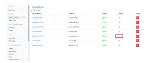
To view the Alarm click on the Device Name, and select the 'Alarms' tab. The alarm page displays the alarm conditions (max and min) as well as the current value of the parameter, the status of the alarm (on or off) and the action for this alarm (edit or delete). The alarms can also be viewed from the Alarm Logs which will be discussed later in the manual.
