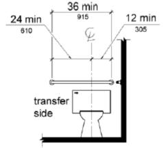
Rear Wall - The rear wall grab bar shall be 36 inches (915 mm) long minimum and extend from the centerline of the water closet 12 inches (305 mm) minimum on one side and 24 inches (610 mm) minimum on the other side.
