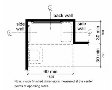
Alternate Roll-In Type Shower Compartments - Alternate roll-in type shower compartments shall be 36 inches (915 mm) wide and 60 inches (1525 mm) deep minimum clear inside dimensions measured at center points of opposing sides. A 36 inch (915 mm) wide minimum entry shall be provided at one end of the long side of the compartment.
